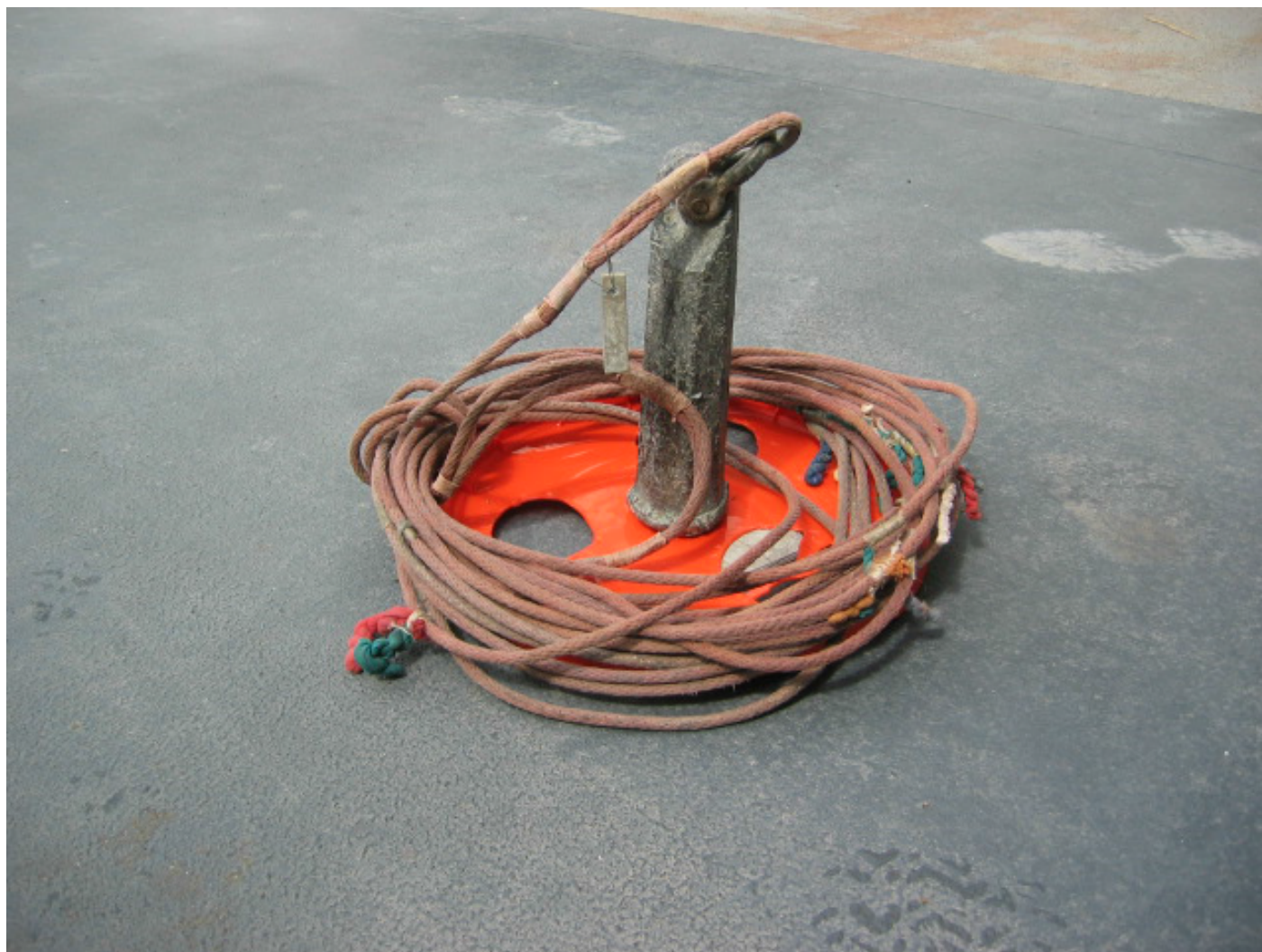
Figure 5: Leadline fitted with custom mud-shoe to limit penetration of soft bottoms.
