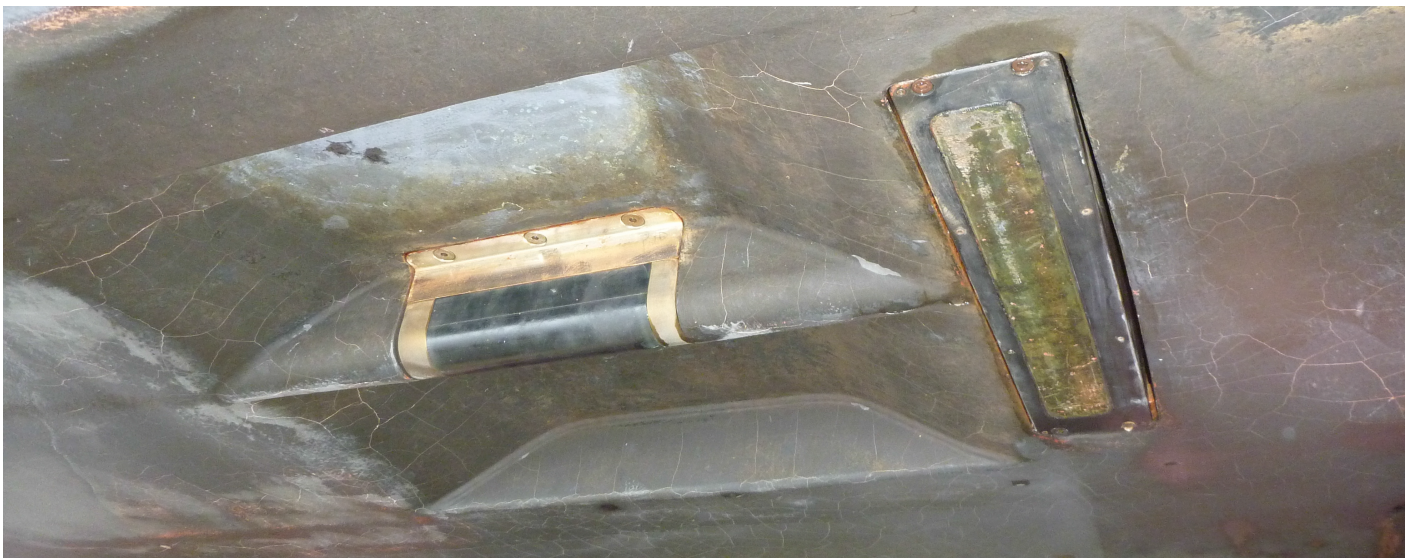
Figure 4: 7125 Housing flush-mounted on hull
