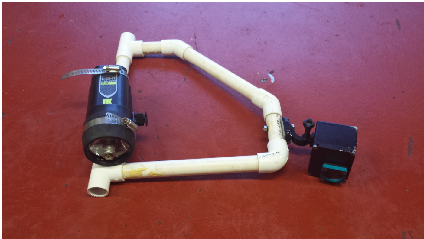
Figure 8: Camera with custom mount allowing for high quality video of the seafloor
