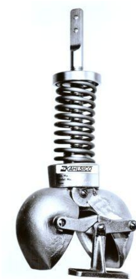
Figure : Snapper type grab sampler used aboard TJ3101 & TJ3102.
