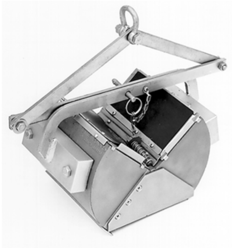
Figure : Ponar style grab sampler used aboard NOAA Ship Thomas Jefferson.
