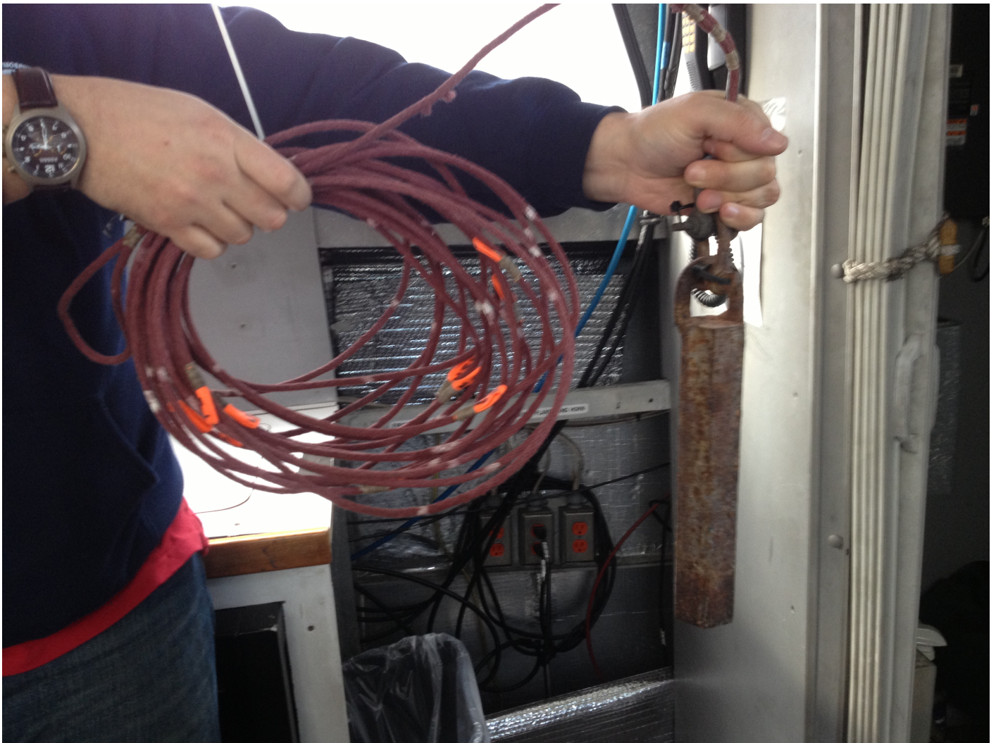
Figure : Lead line used aboard Thomas Jefferson and her survey launches
