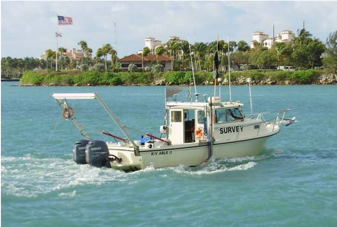
Figure 1. R/V Able II in multibeam/SSS configuration.
