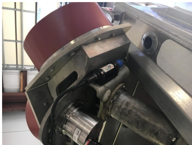
Figure 6: AML Micro•X Sensor Mobilized on a Kongsberg 2040C
