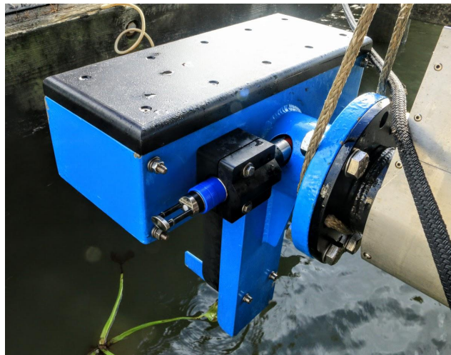
Figure 5: AML Micro•X Sensor Mobilized on an R2Sonic 2024
