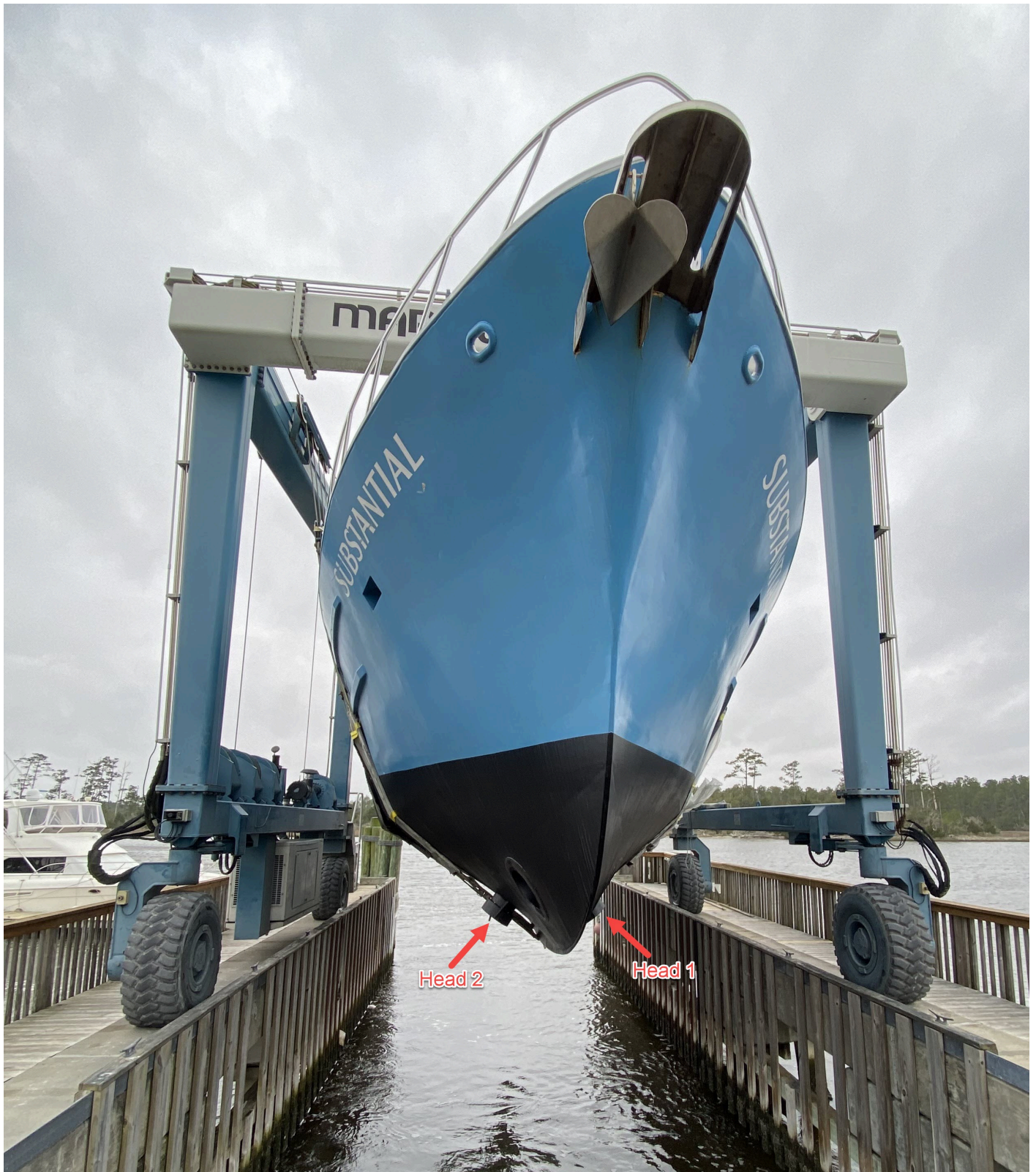
Figure 5: Kongsberg EM2040C dual-head sonar hull mounted on the R/V Substantial with each transducer labeled
