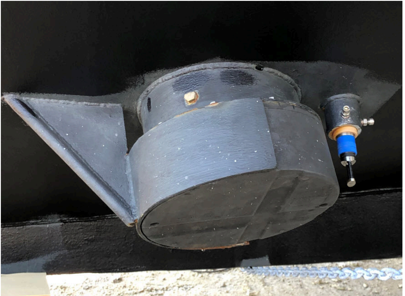
Figure 6: Kongsberg EM2040C hull mount on the R/V Substantial
