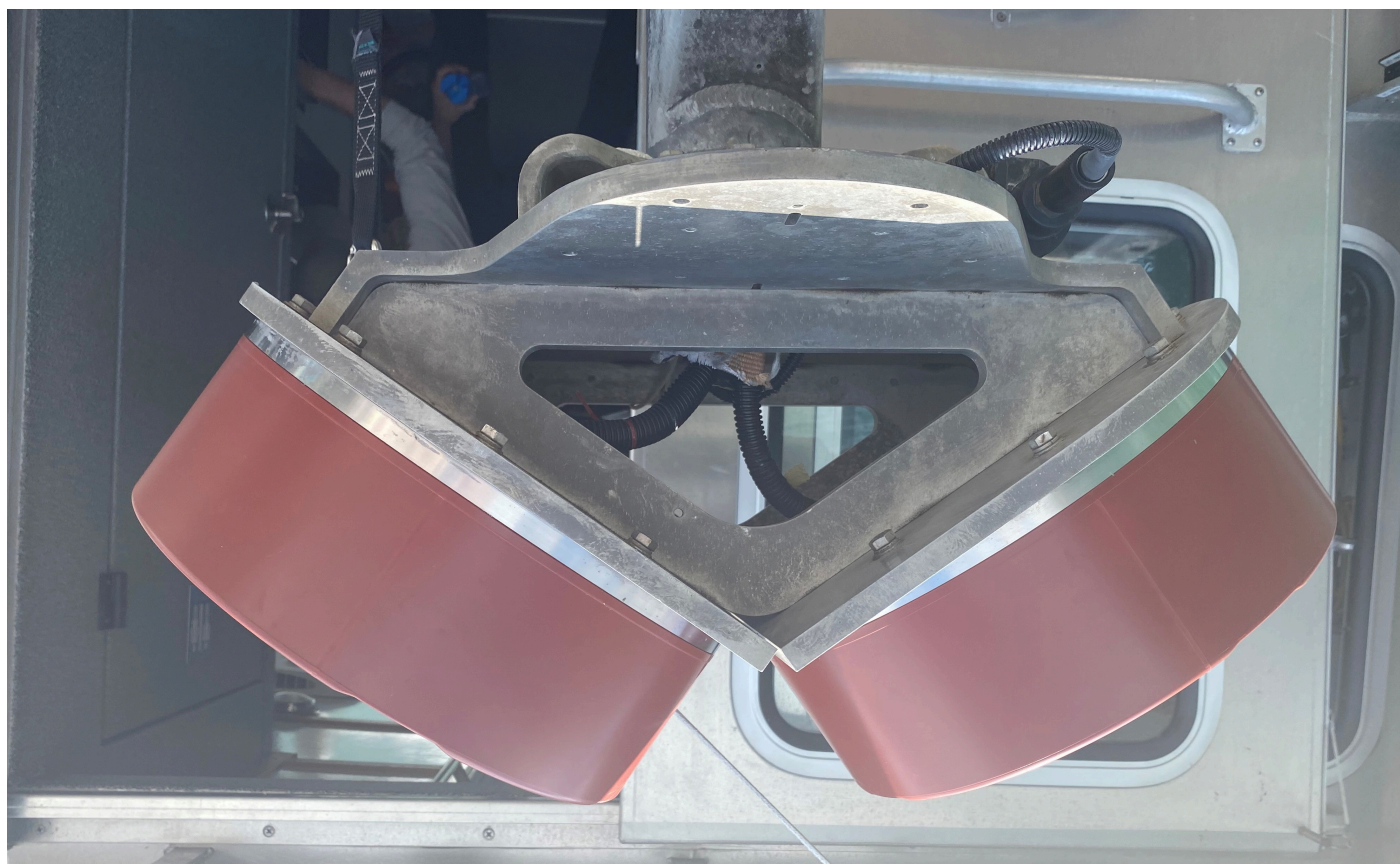
Figure 4: Kongsberg EM2040C dual-head sonar on a pole mount
