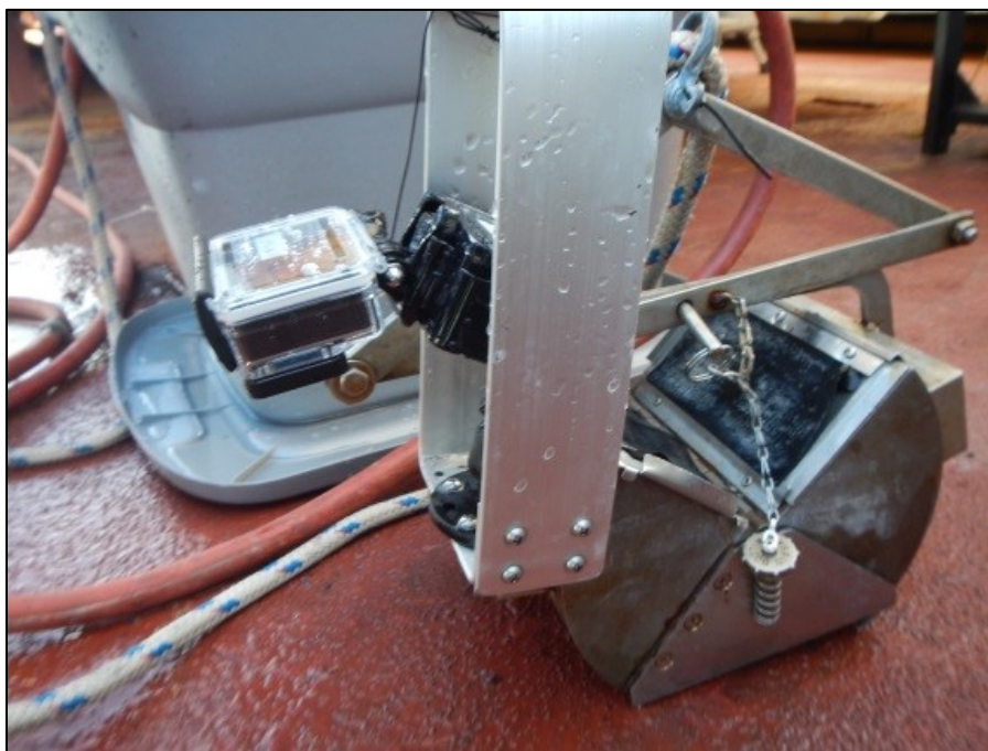
Figure A-3: GoPro Camera Mounted on Petite Ponar Grab
