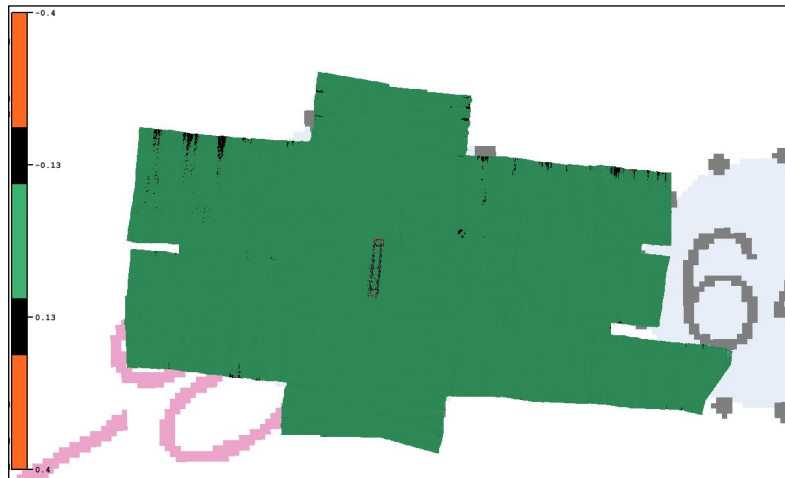
Figure 11: Vessel to Vessel Comparison (Difference Surface)
