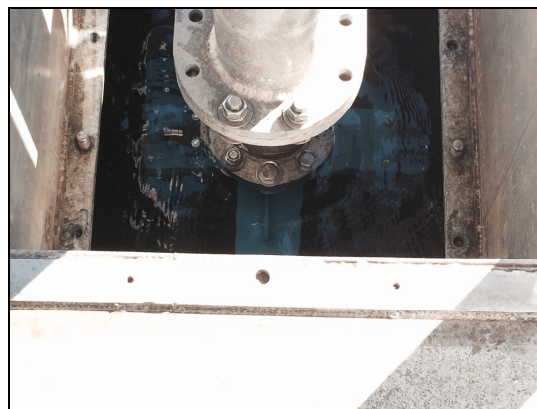
Figure 4: R2Sonic 2024 - M/V Jab - Midway Through Moonpool Deployment
