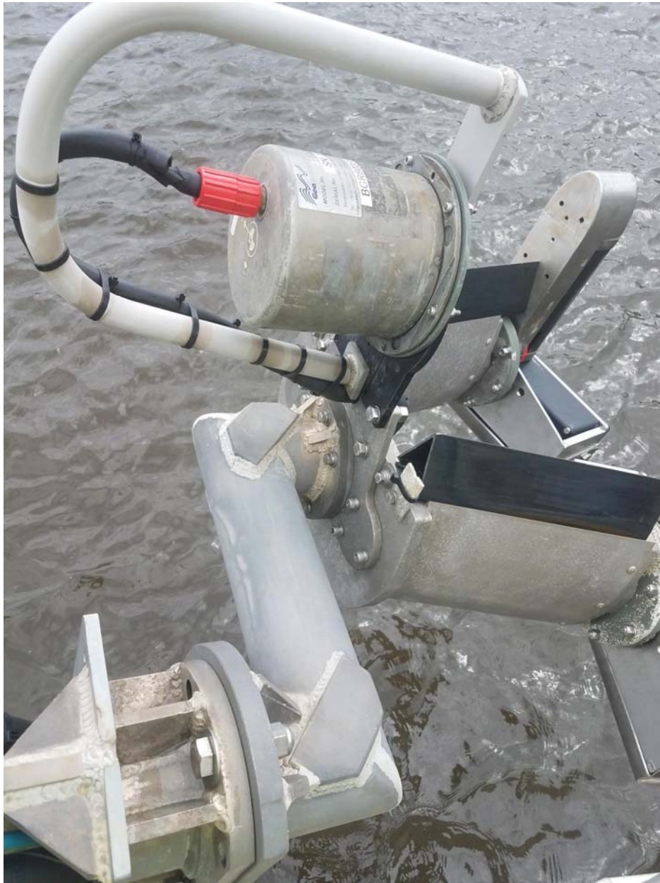
Figure 3 M/V Pelagos Dual 7125 with Underwater IMU
