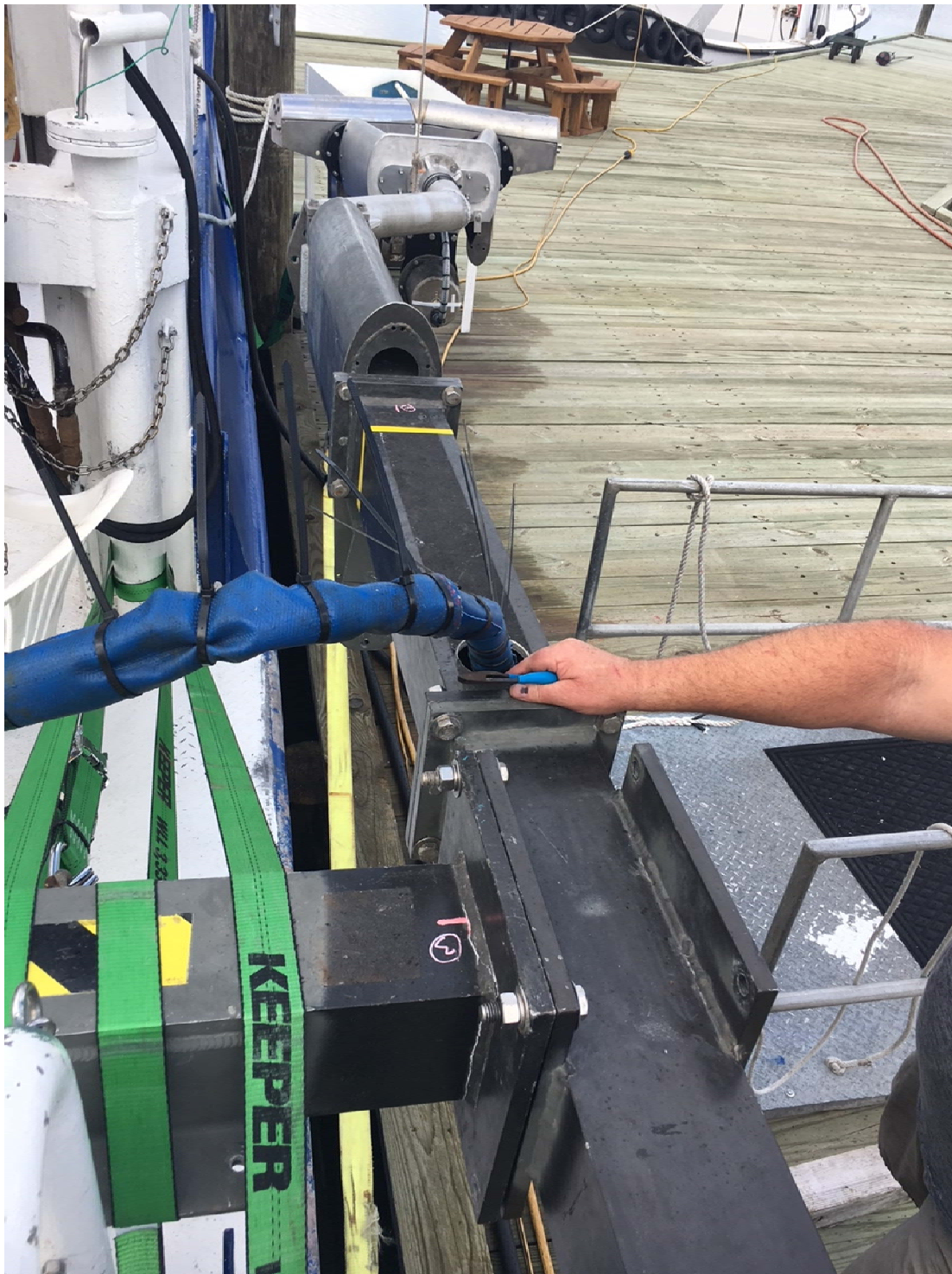
Figure 7 R/V Acadiana Dual 7125 with Underwater IMU
