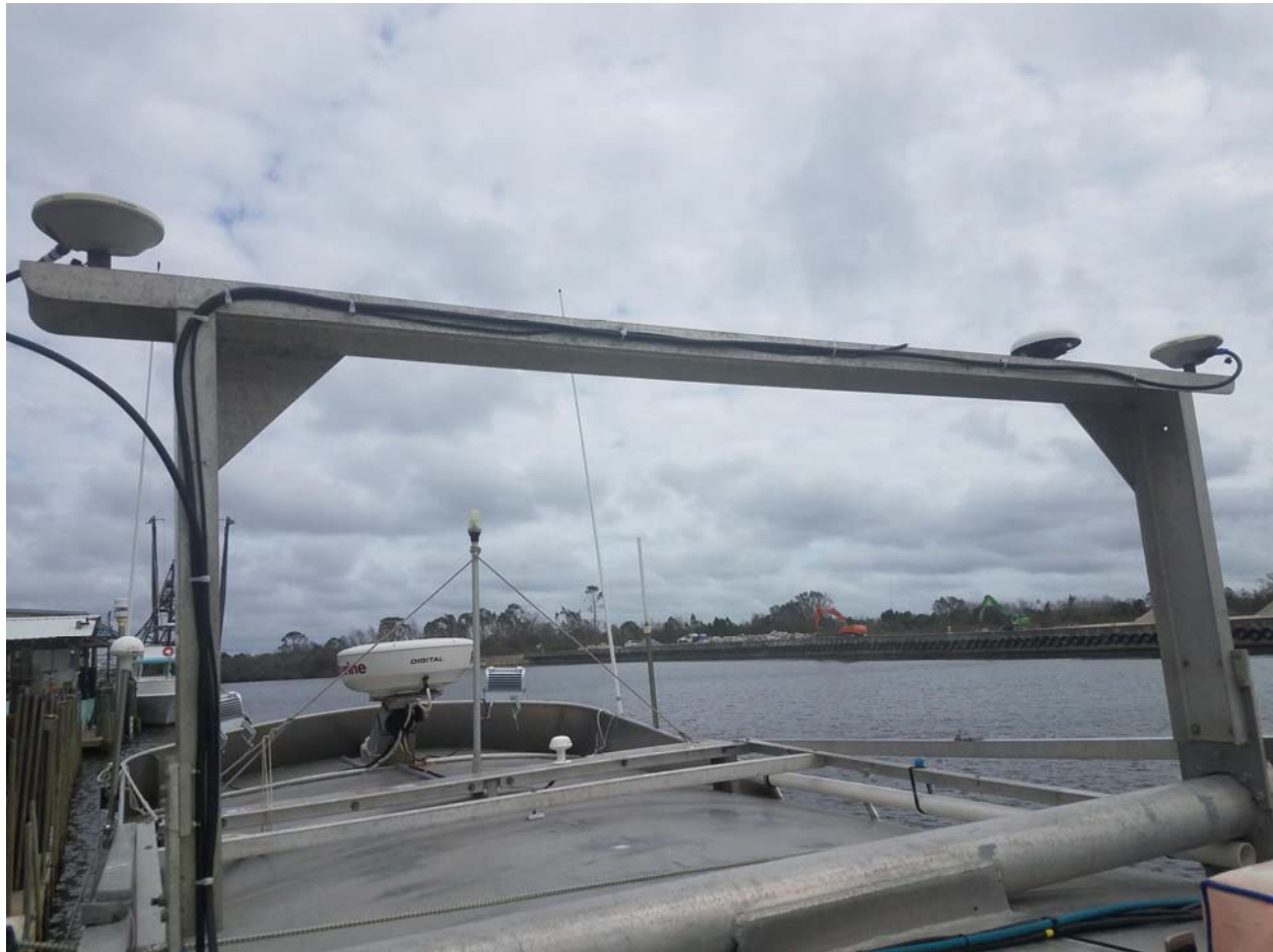
Figure 4 M/V Pelagos Trimble L1/L2 Antennas
