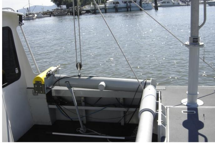
The Reson 8125 forms 240 beams each of which has a  $0.5^\circ$  across-track beam footprint for a maximum total swath width of  $120^\circ$ . Each beam has an along-track resolution of  $1^\circ$ . The ping rate is nominally 20-40 Hz, but may vary according to operating conditions. The Reson 8125 sonar is capable of bottom detection in depths from 3-120m.
