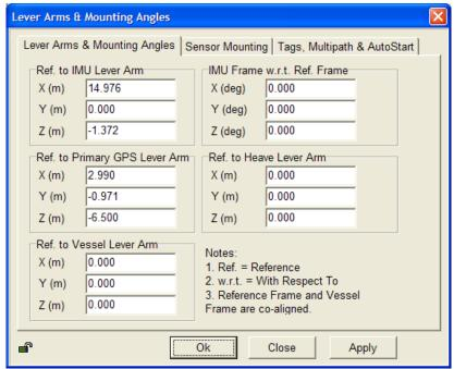
Illustration No. 5: POSMV GPS and IMU lever arms from the CRP.
