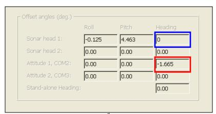
Illustration No. 7. Patch test results from June 30<sup>th</sup>, 2011 and where they were entered in SIS. When the heading is entered under Attitude 1, COM2, it is corrected for in real-time (red box). However, the November 11<sup>th</sup> heading value was entered in Sonar head 1 where it is not corrected for in real-time (blue box), and therefore was corrected for in the CARIS vessel file.
