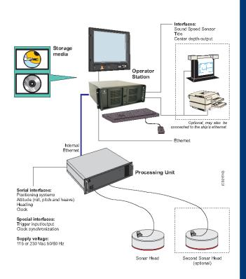
Typical system configuration with desktop Operator Station, Processing Unit and one or two Sonar Heads.
