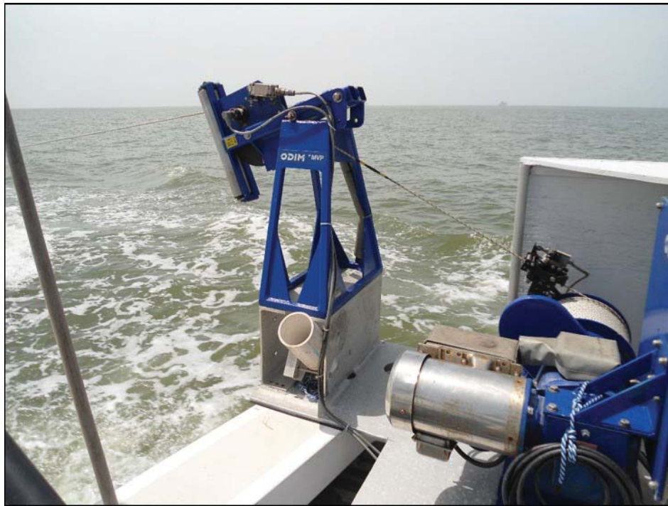
Figure 7. ODIM MVP30 as mounted on the port quarter of the R/V Ocean Explorer .
