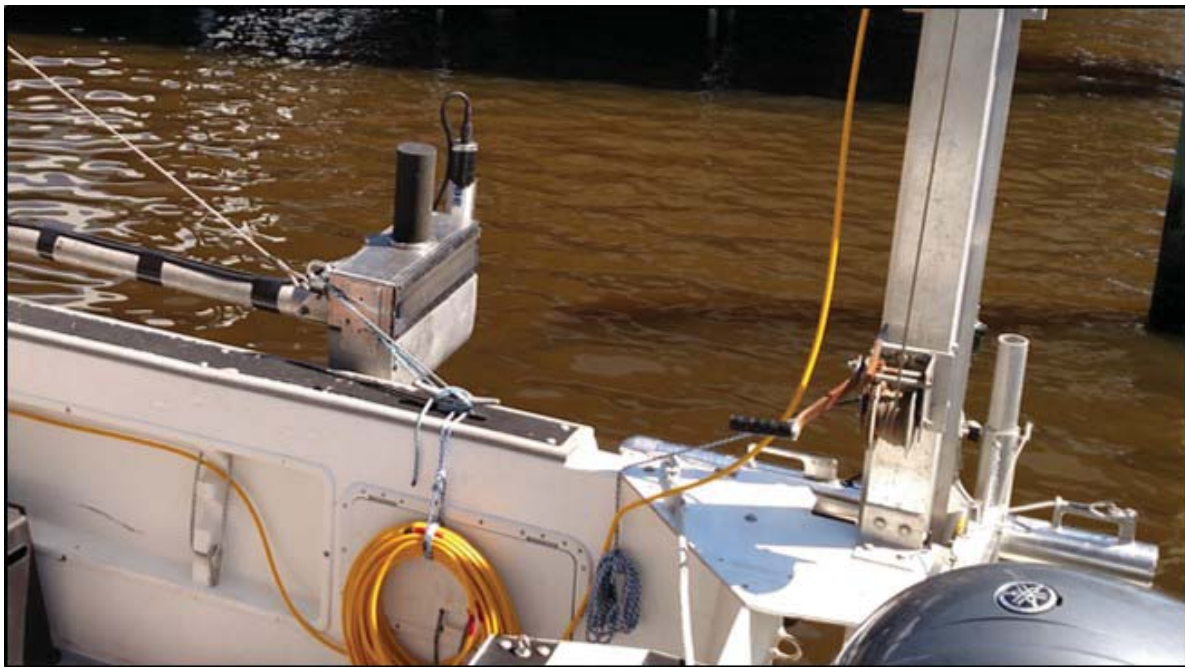
Figure 6. Pole-mounted Reson 8125 transducer (with custom bow faring) as configured on the R/V Osprey for Project OPR-K354-KR-17. Note the Sea-Bird SBE37 surface sound speed sensor attached to the outboard side of the multibeam transducer. Also note the pole mounted SSS deployment post and aft end of EdgeTech 4125 SSS fish on the right side of this image.
