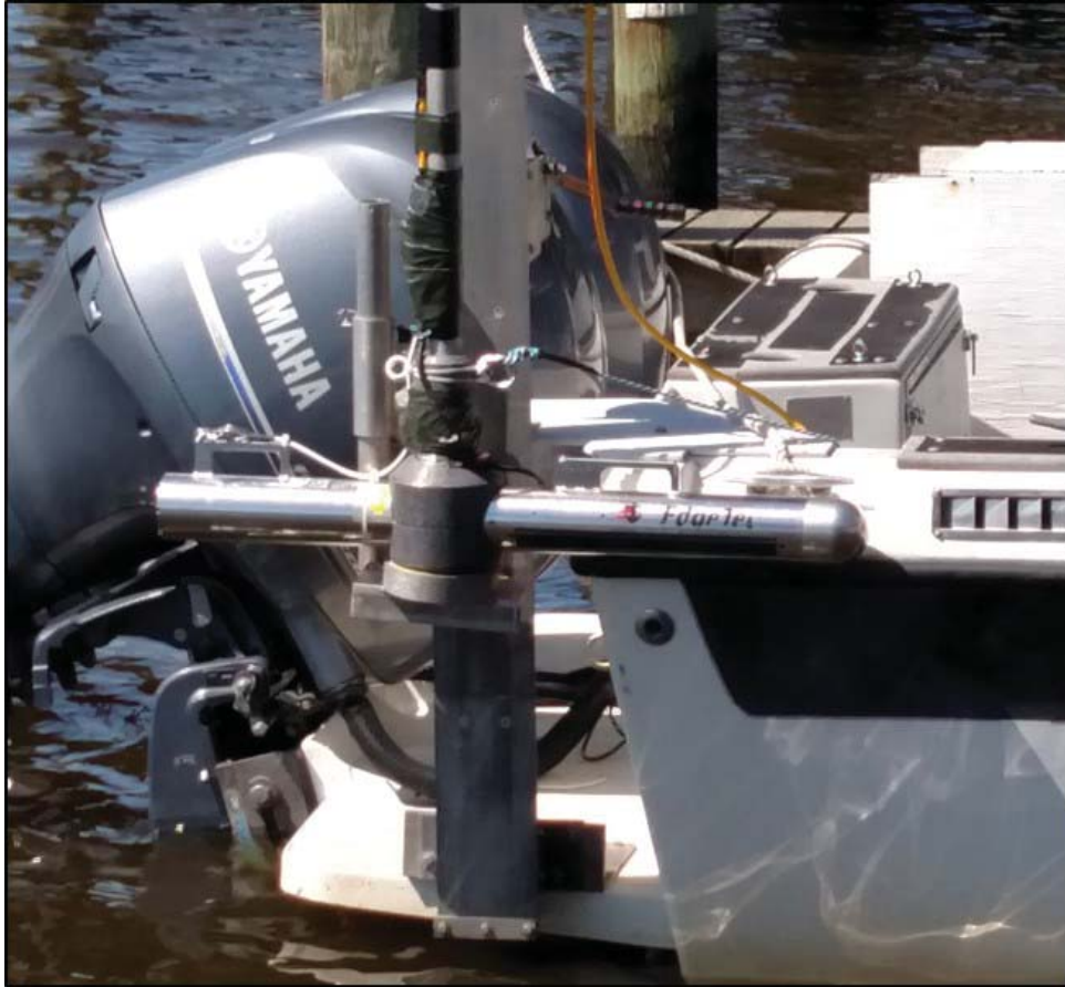
Figure 4. Pole-mounted EdgeTech 4125 SSS transducer as configured on the R/V Osprey for Project OPR-K354-KR-17. In this photo the SSS is resting in its transit cradle.
