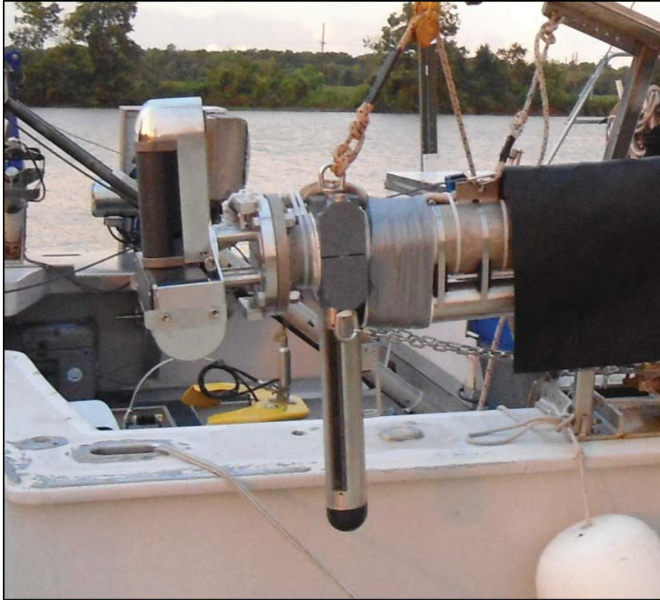
Figure 3. Pole-mounted EdgeTech 4125 SSS transducer as configured on the R/V Ocean Explorer for Project OPR-K354-KR-17. The AML Micro X surface sound speed sensor is located within the multibeam bow fairing. Note that the SSS transducer module (pointing down in this photo) is separated from the electronics module which is secured parallel to the forward side of the transducer pole. A Reson 7125 transducer is mounted to the bottom of the pole in this photo.
