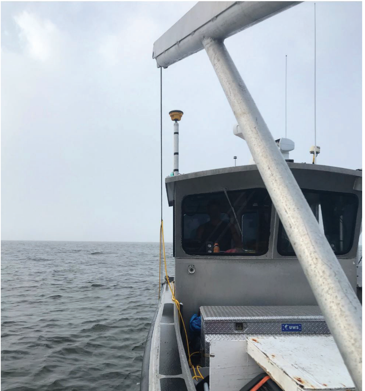
Figure 8: Edgetech 4200 SSS Towpoint on R/V H.F. Stout
