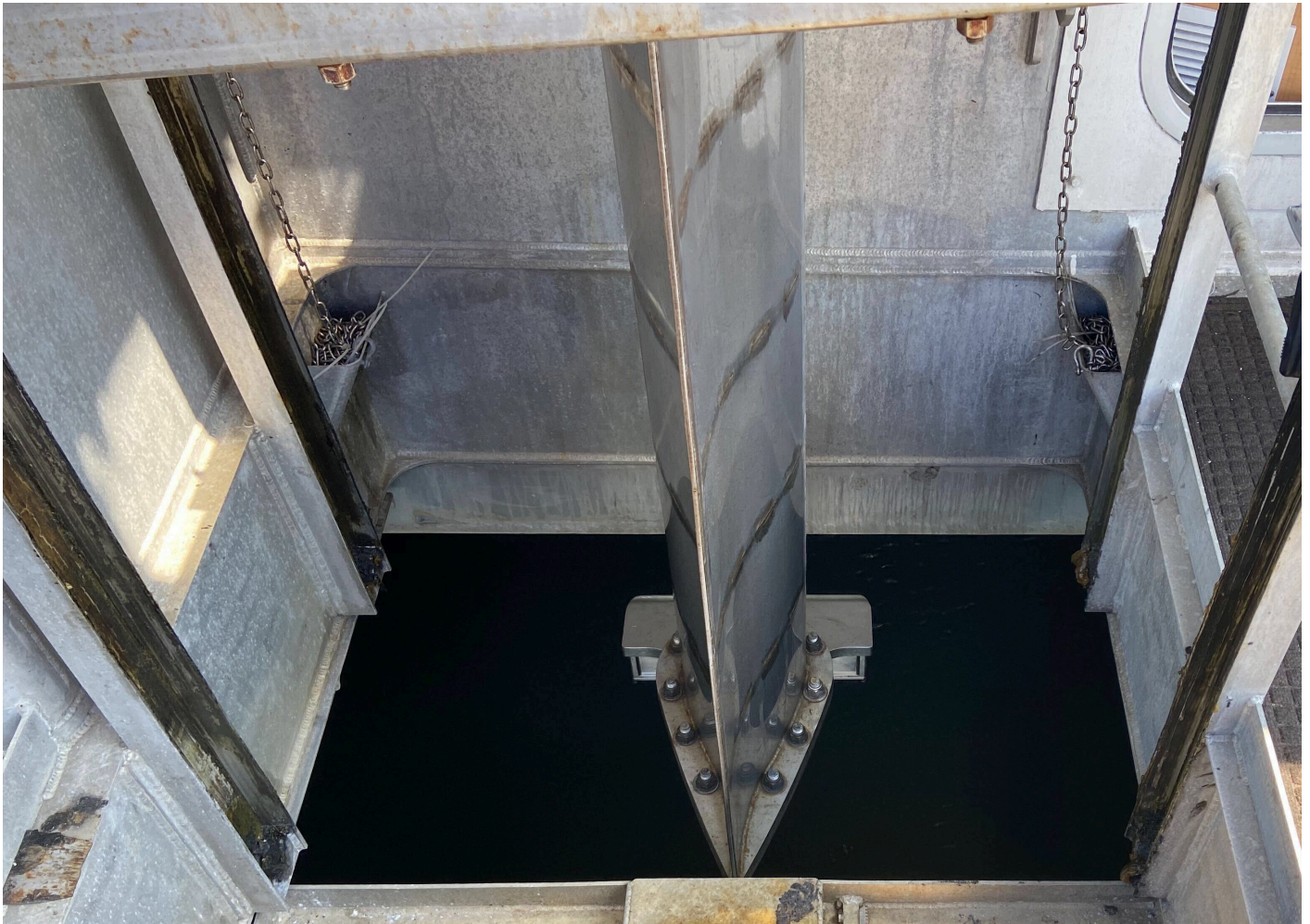
Figure 3: Blake Retractable Moon Pool and Center-Pole Mount
