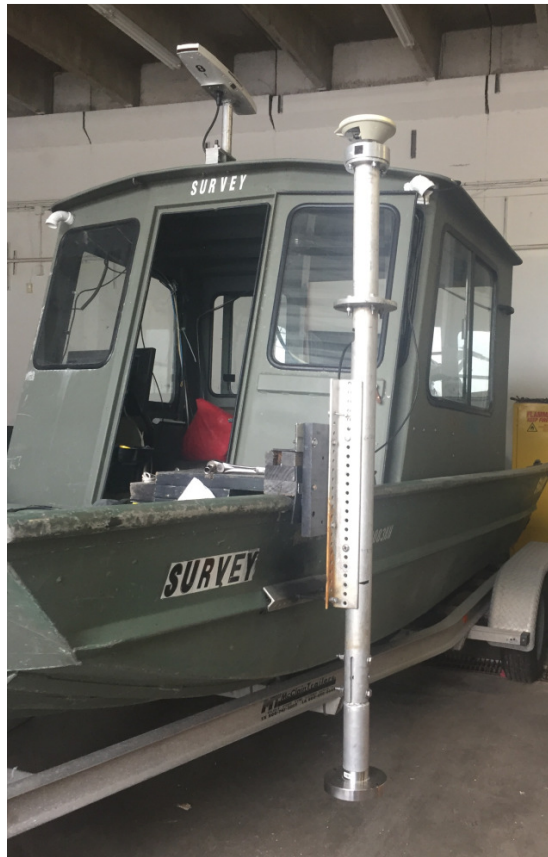
Figure 6 – Sea Ark on trailer, with port-bow mounted SBES
