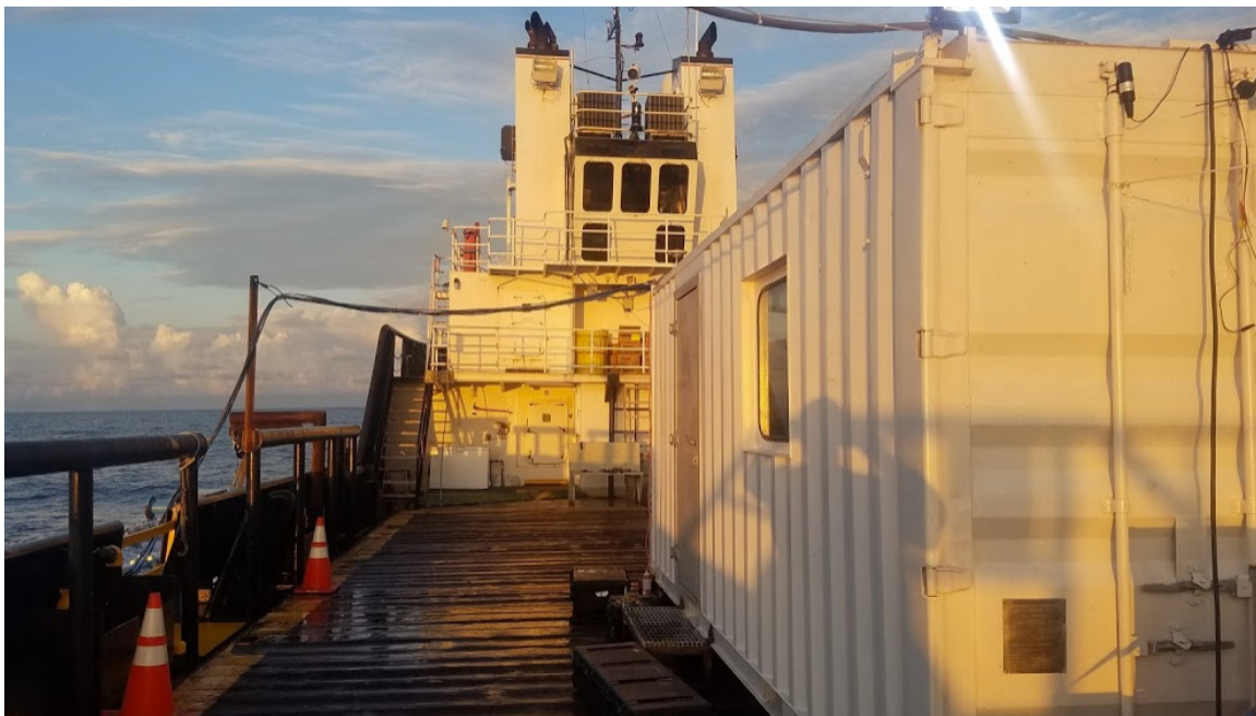
Figure 5 R/V Bunny Bordelon back deck showing offshore Conex. MBES pole is deployed on the port side, indicated by aerial MBES cables
