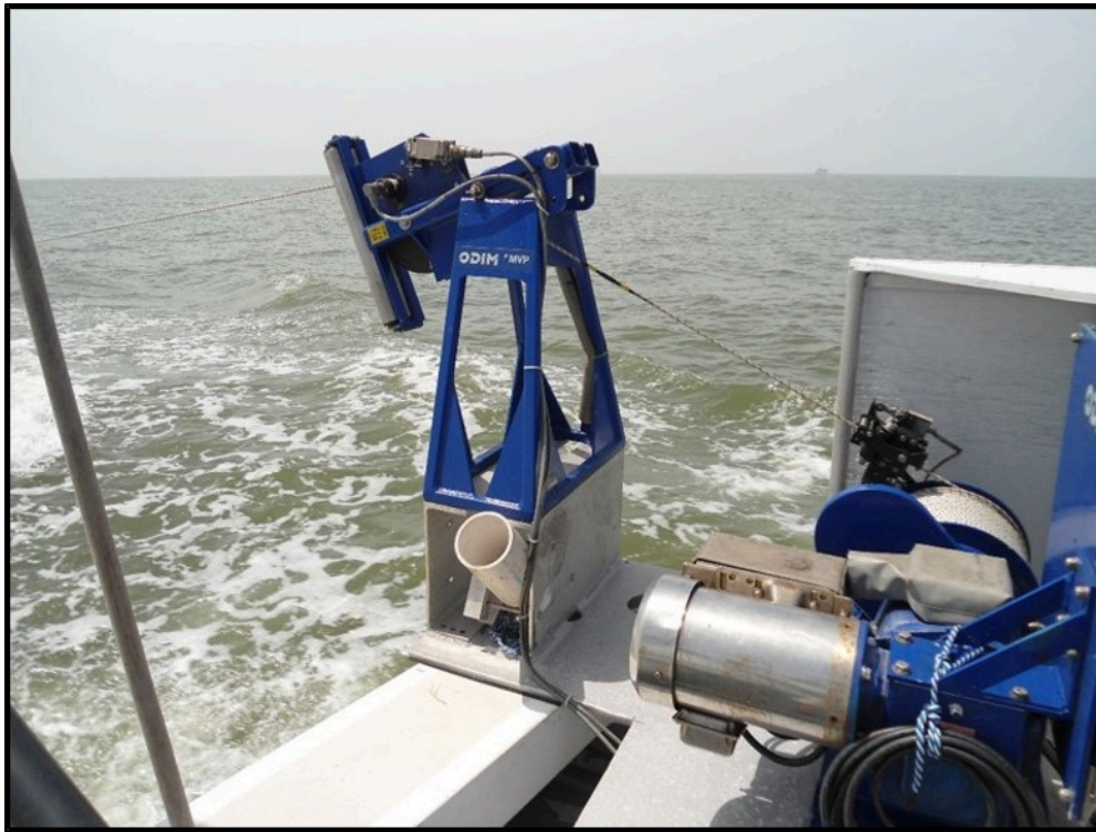
Figure 10: MVP 30 Moving Vessel Profiler mounted on the port quarter of the R/V Ocean Explorer
