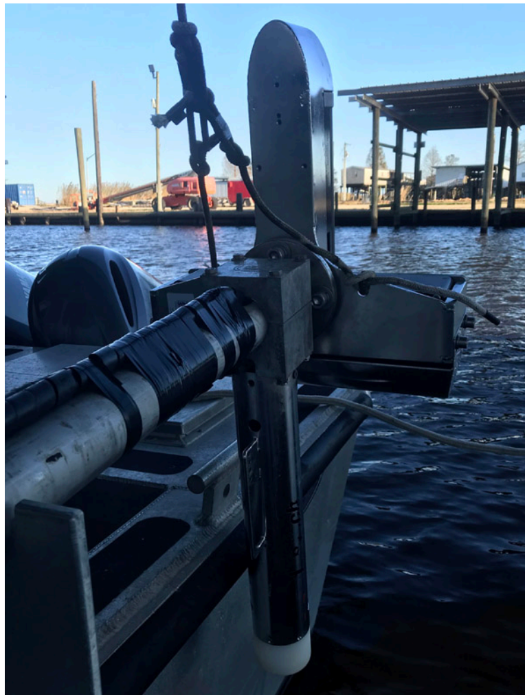
Figure 7: Edgetech 4125 SSS towfish mounted on the transducer pole of the R/V H.F. Stout
