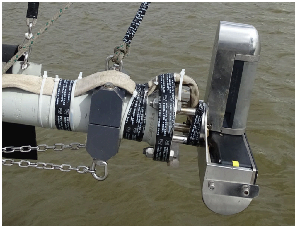
Figure 3: Seabat 7125 SV2 transducer mounted on the R.V. Ocean Explorer transducer pole.
