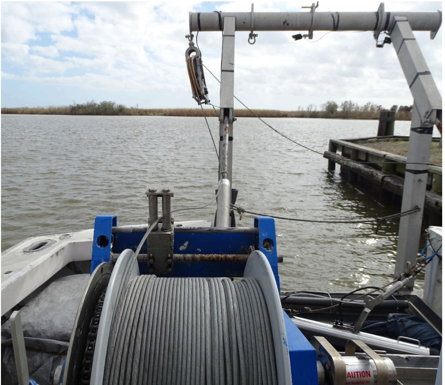
Figure 6: Electric SSS winch and cable-counting sheave aboard the R/V Ocean Explorer
