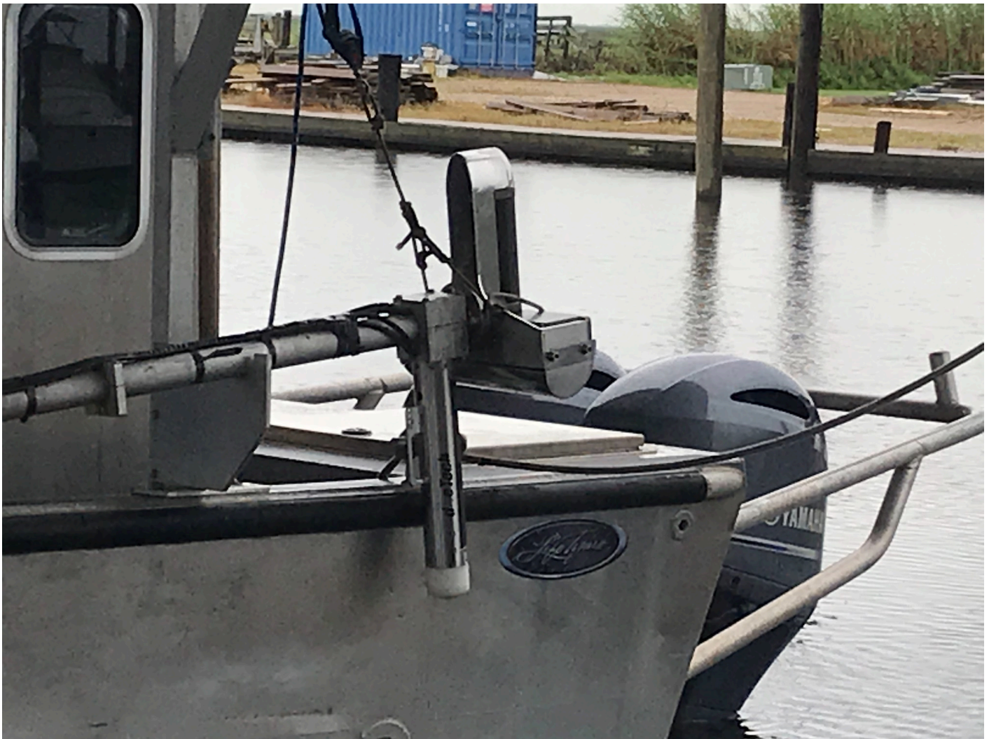
Figure 4: Seabat 7125 SV2 transducer mounted on the R.V. H.F. Stout transducer pole.
