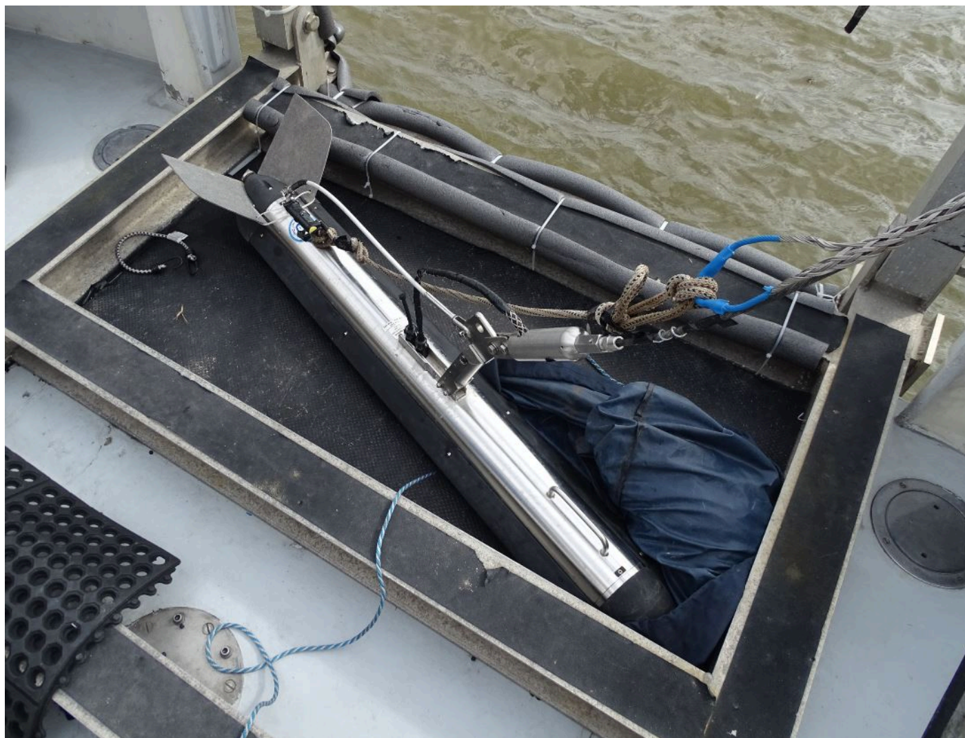
Figure 5: Edgetech 4200 MP SSS towfish aboard the R/V Ocean Explorer
