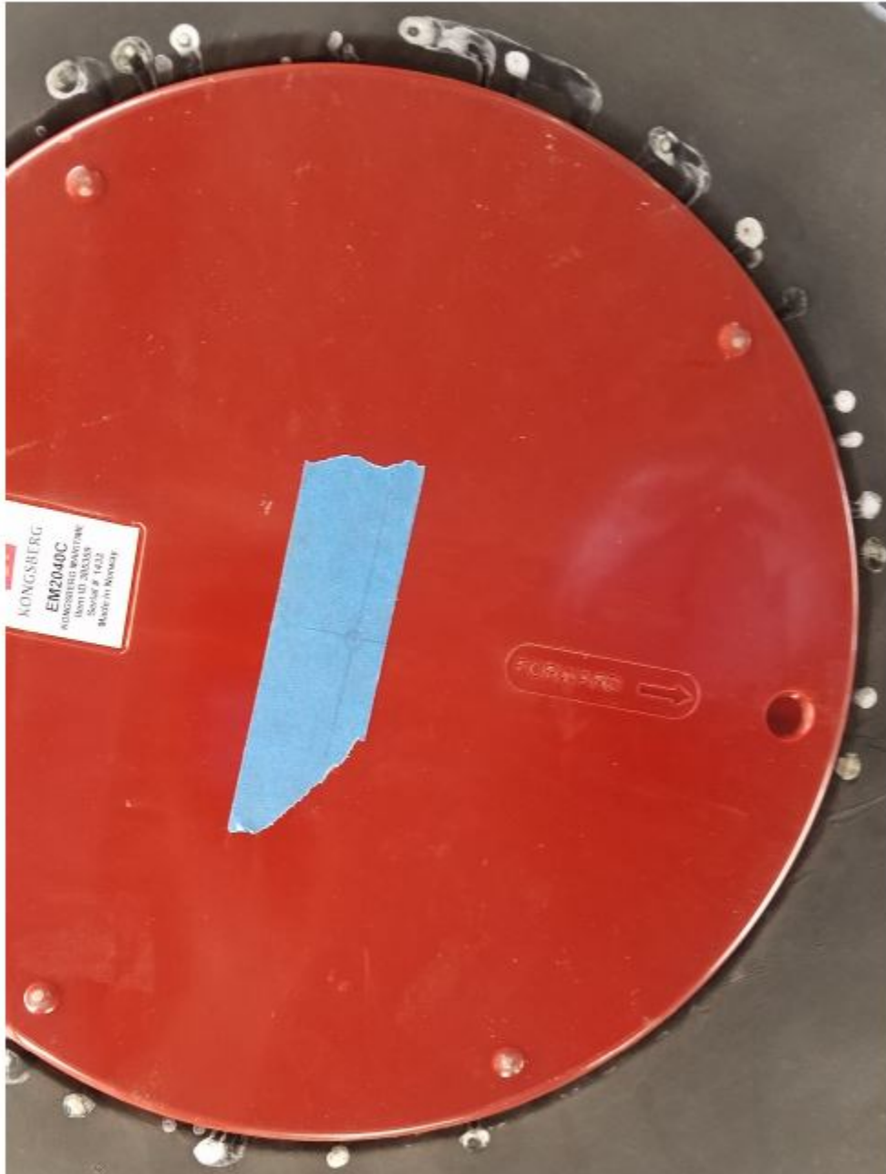
Figure 16: EM2040C Vessel Reference Point
