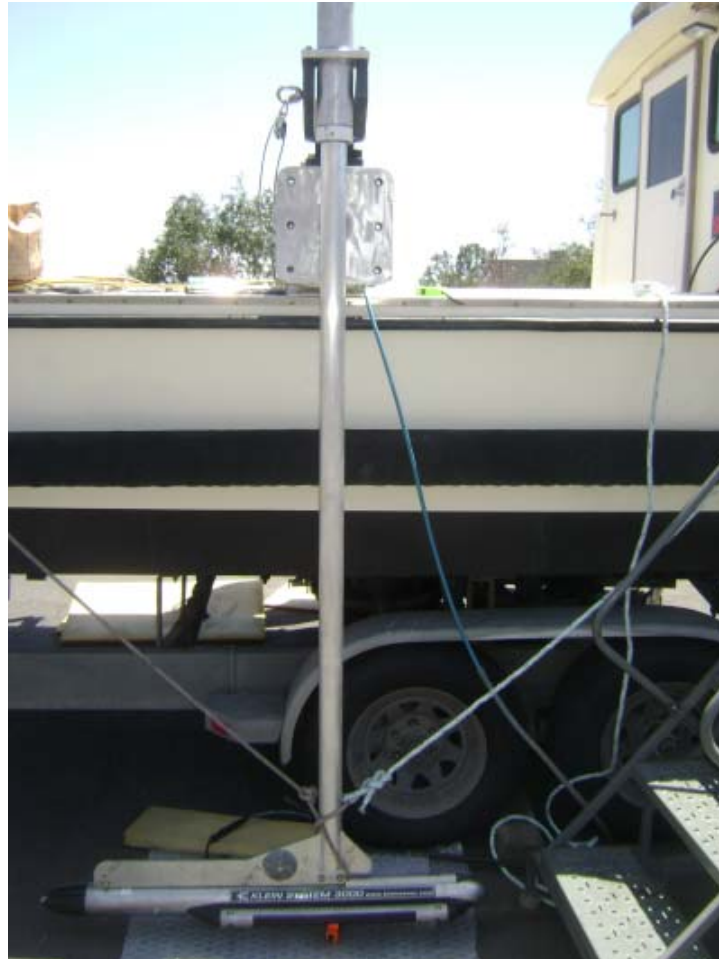
Figure 7 – Pole mounted SSS on Locator
