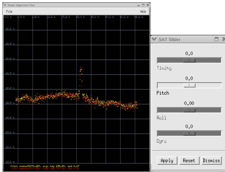
Figure C-10. SAT Tool, Depth vs. Distance Plot Depicting 0.00 Pitch Bias
