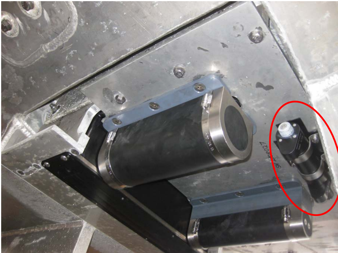
Figure 7: SVP 71 sound speed unit (right) and a Reson 7125
