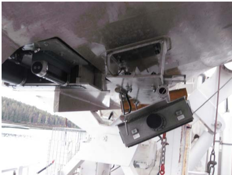
Figure 5 : Reson 8125 Tilted Head Mounted on Launch 2808
