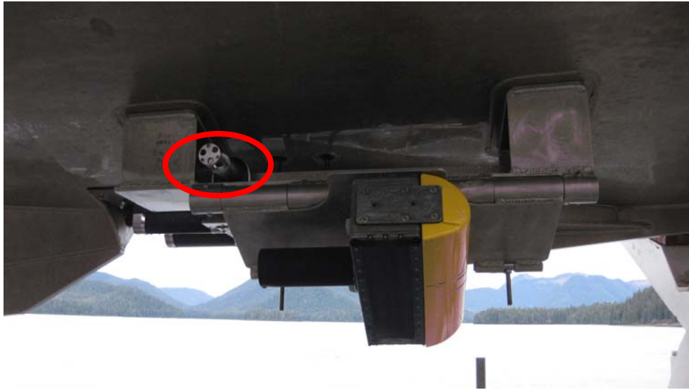
Figure 8 : Odom Digibar and Reson 8125 Tilted Head on Launch 2808
