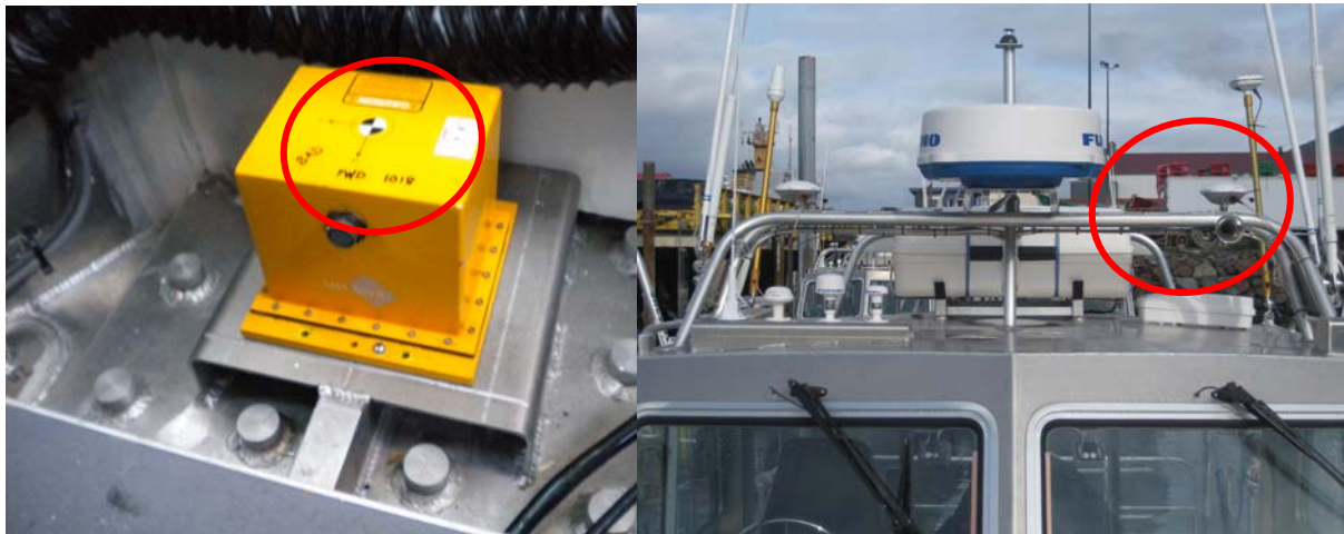
Figure 9: Vessel Reference Point (Top of POS MV IMU) & Primary GNSS Antenna (port side).
