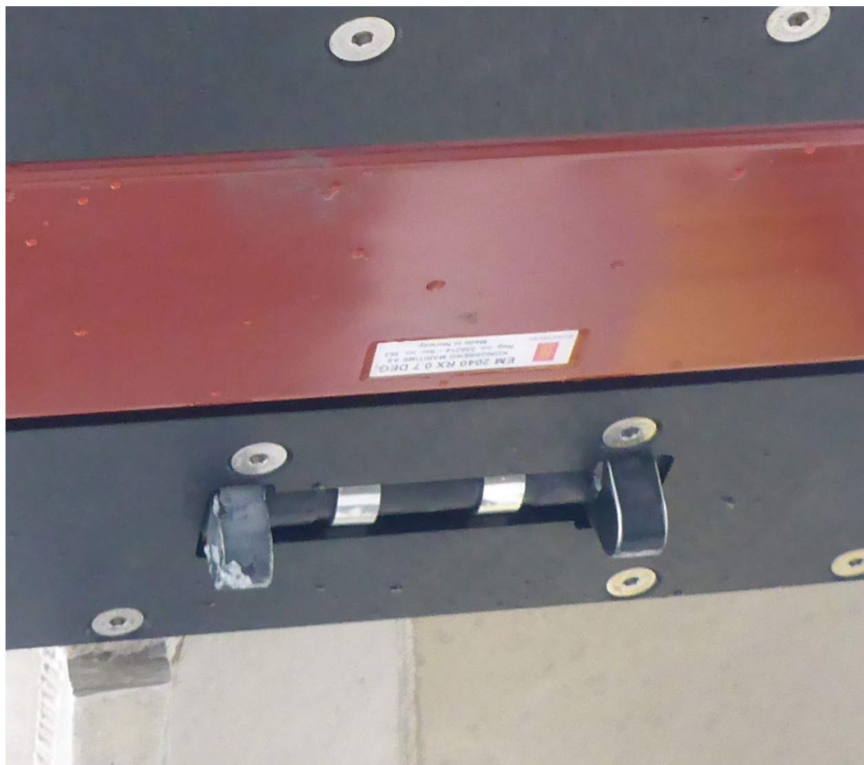
Figure 13: A SVP 71 mounted just aft of a Kongsberg multibeam transducer on a survey launch.
