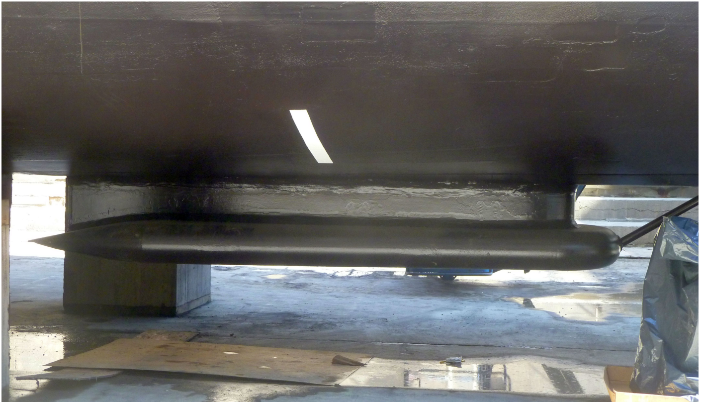
Figure 8: Kongsberg EM710 sonar transducer housing on Rainier (S221).
