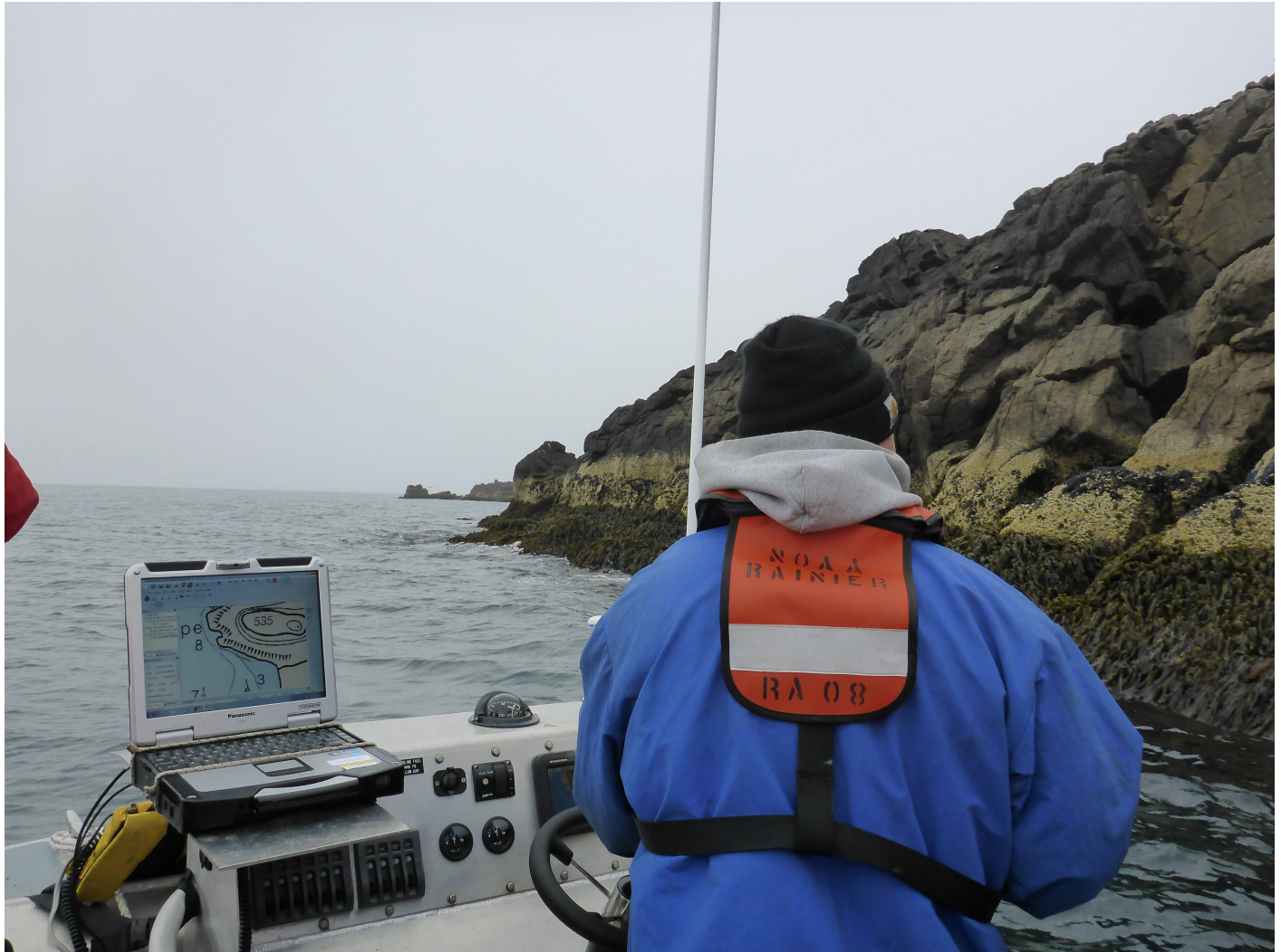
Figure 16: Survey skiff RA7 collecting the along-shore buffer line using a Trimble GPS backpack system connected to an external battery and a Toughbook computer.
