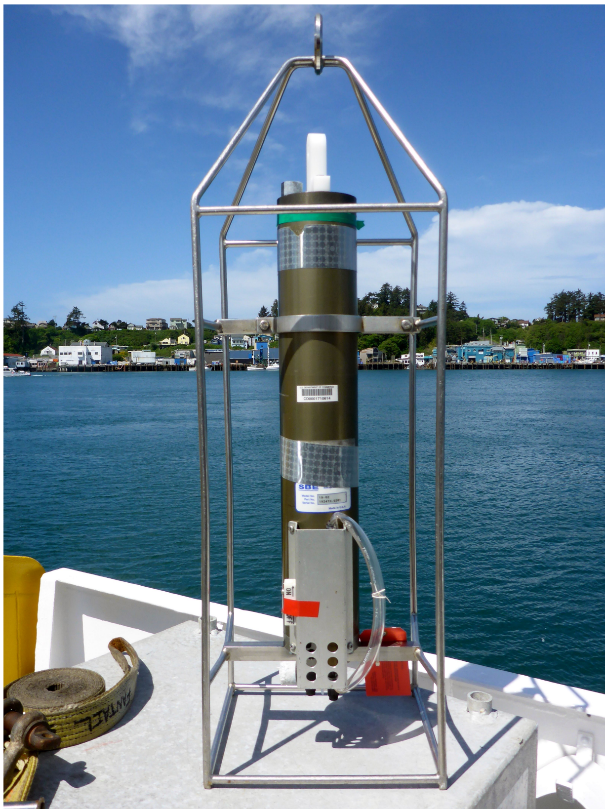
Figure 10: The SEACAT SBE 19 profiler. Note the band of electrical tape around the housing at the top of profiler marking this as the "green" CTD.
