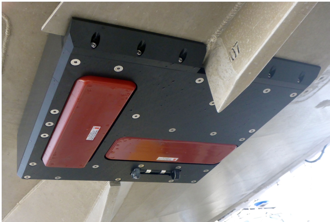
Figure 9: The Kongsberg EM 2040-07 mounted on survey launch 2803.
