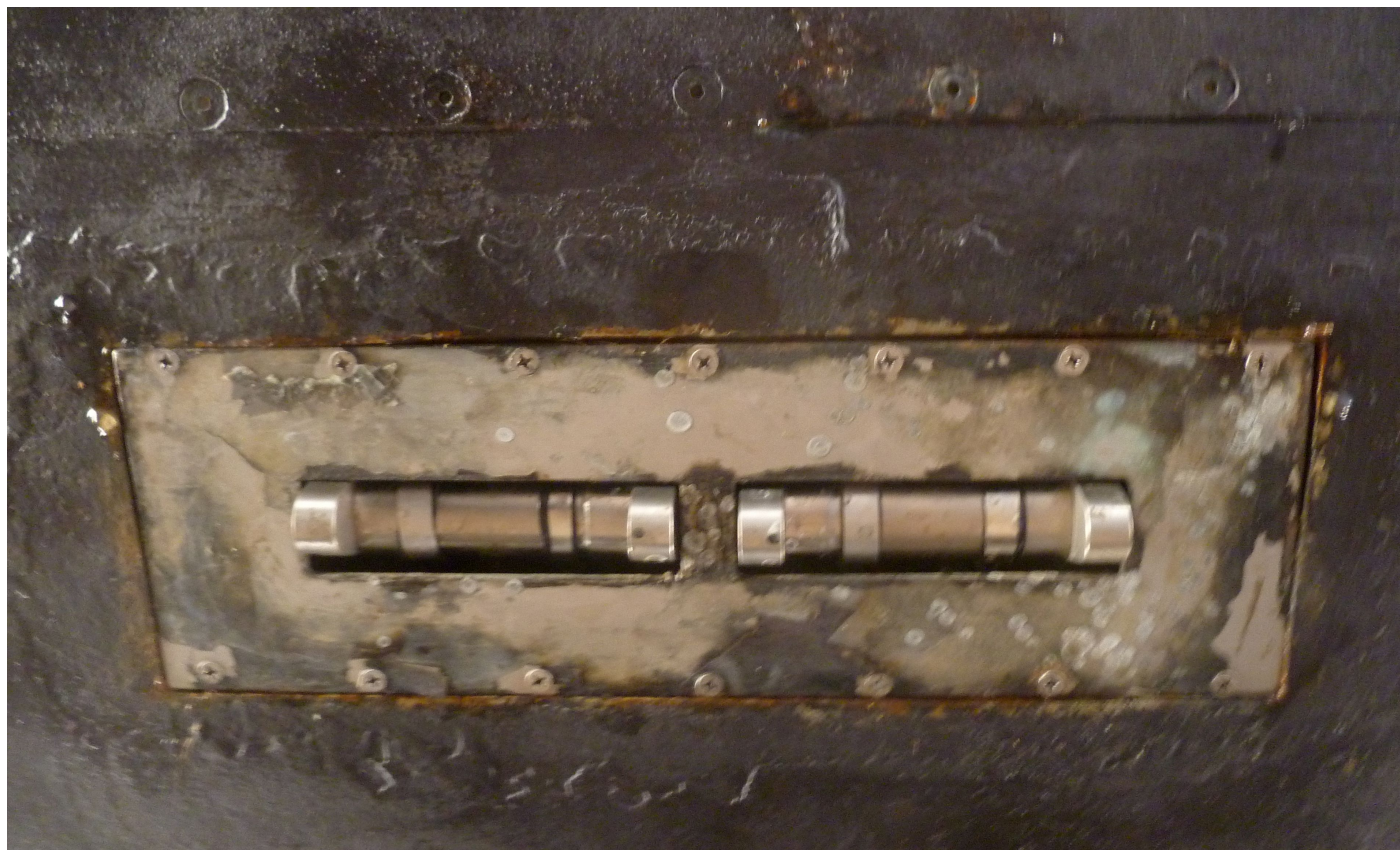
Figure 12: Dual SVP 70s mounted in Rainier's multibeam sonar transducer gondola.
