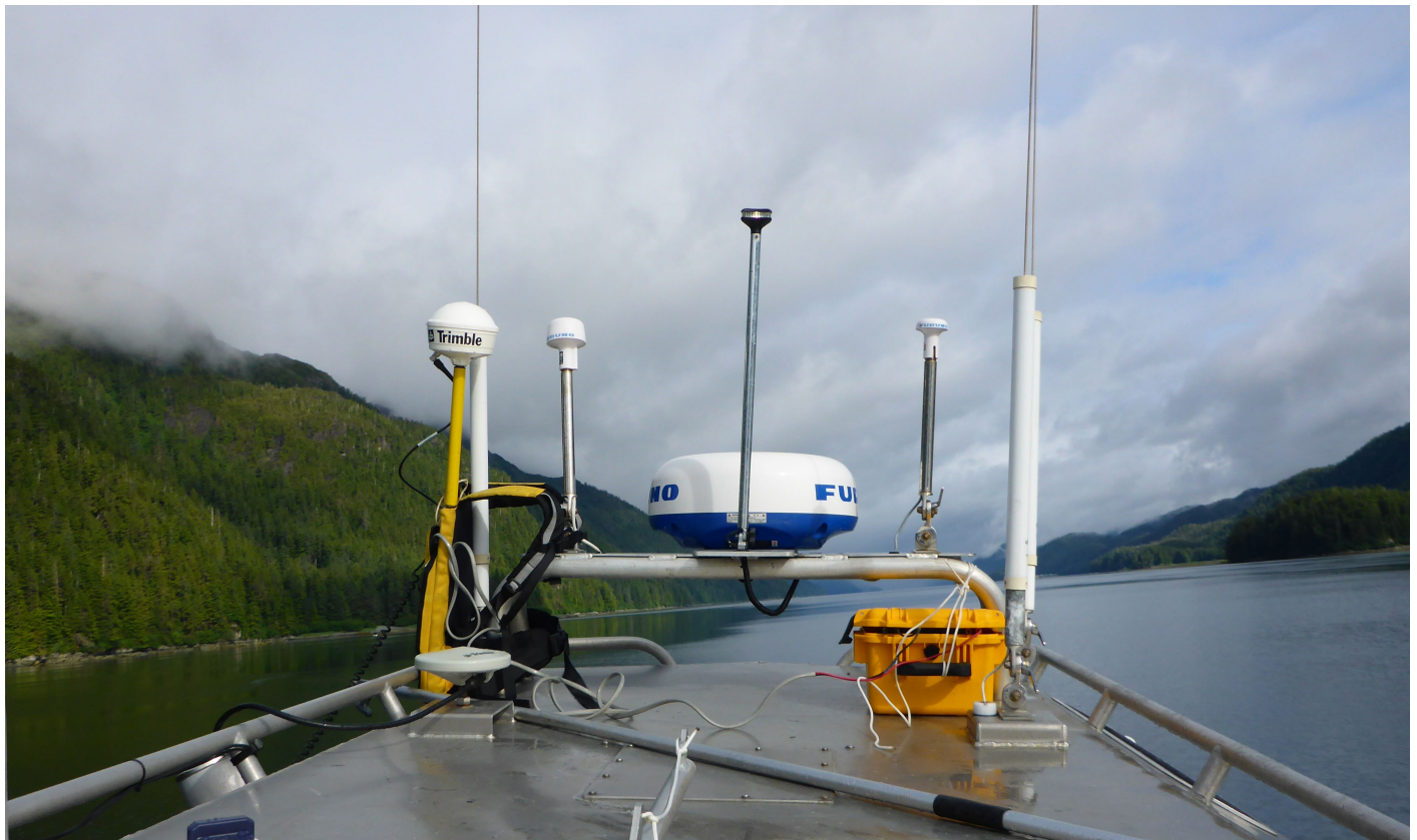
Figure 12: A Trimble “backpack” GPS system and battery tied down on the roof of RA2 (2701) during shoreline verification.
