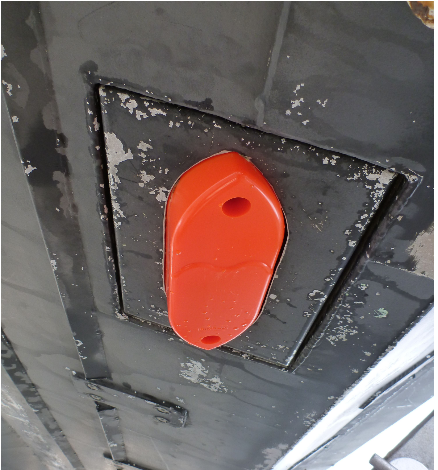
Figure 11: The Simrad 50/200 Combi D transducer as mounted on 2701 for the Teledyne Odom Hydrographic Echotrac CV200 hydrographic echo sounder.
