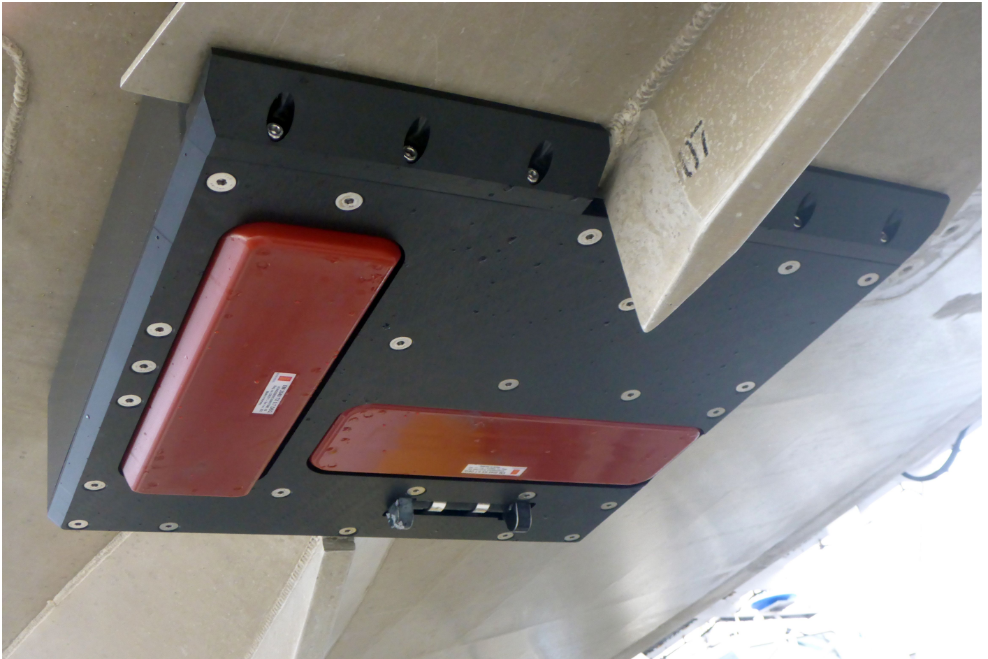
Figure 10: The Kongsberg EM2040-07 mounted on survey launch 2803.
