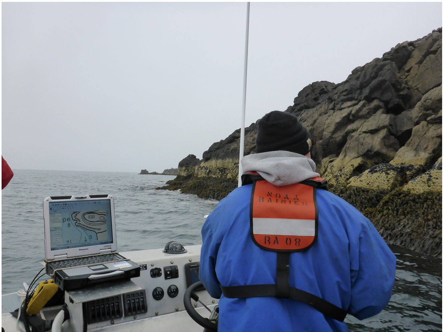
Figure 18: Survey skiff RA7 collecting the along-shore buffer line using a Trimble GPS backpack system connected to an external battery and a Toughbook computer.
