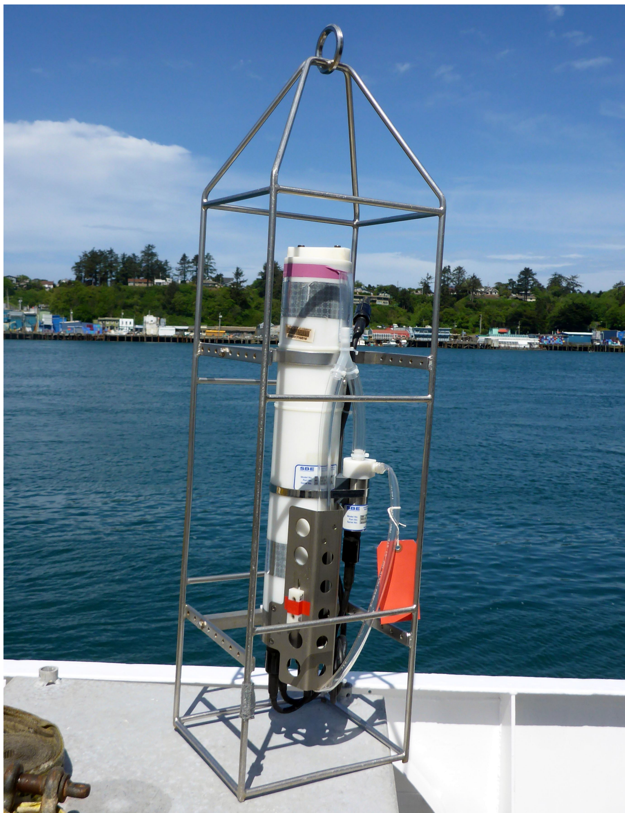
Figure 14: The SBE 19plus SEACAT profiler. Note the band of electrical tape around the housing at the top of profiler marking this as the "purple" CTD.
