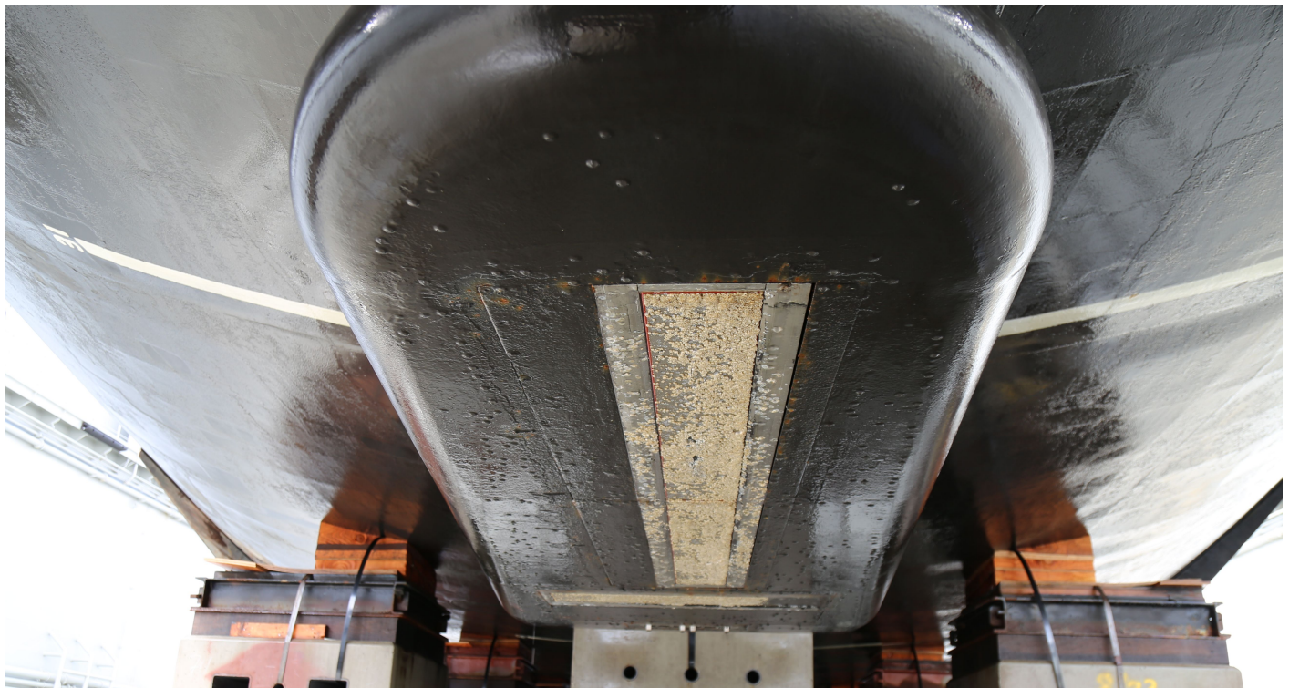
Figure 9: Kongsberg EM710 sonar transducer housing on Rainier (S221).
