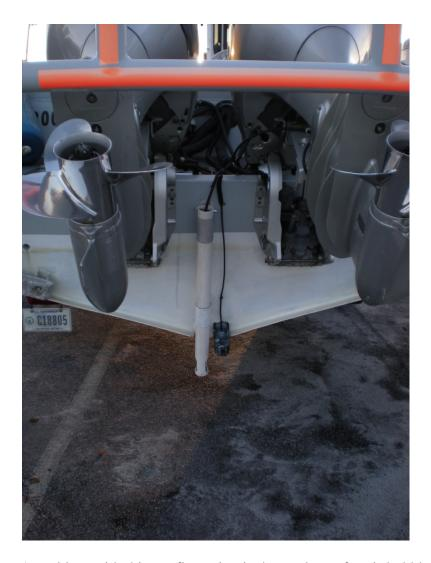
A problem with this configuration is the tendency for air bubbles (turbulence) and debris, mostly floating eel grass, to become trapped in the PVC tube, leading to large errors in the sound velocity. This in turn causes the multibeam to incorrectly steer the incoming pings, seen as large "frowns" in the bathymetry. Data exhibiting this problem are noted, and data are re-acquired over the problem areas.
