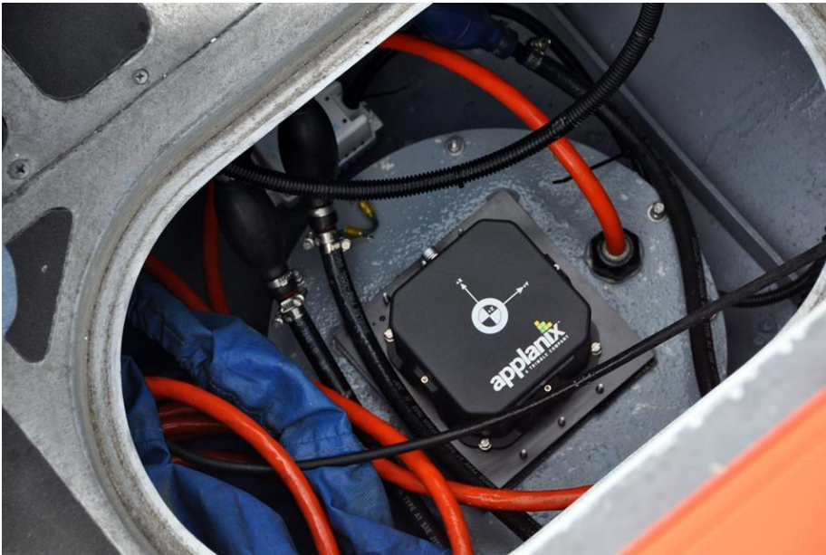
Figure 6: IMU mounted in hatch directly above the multibeam transducer.
