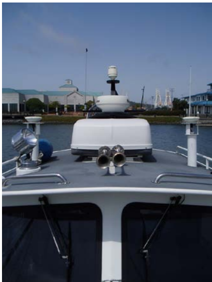
Figure 5: View of top of house on Launch S3003. Center GPS antenna is used by Trimble SPS361 receiver, and two lower antennae are used by the POS/MV V5.
