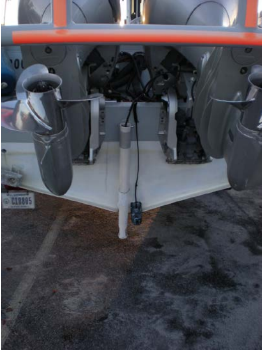
Figure 2: S3003 AML/Digibar mount and protective PVC sheath.
