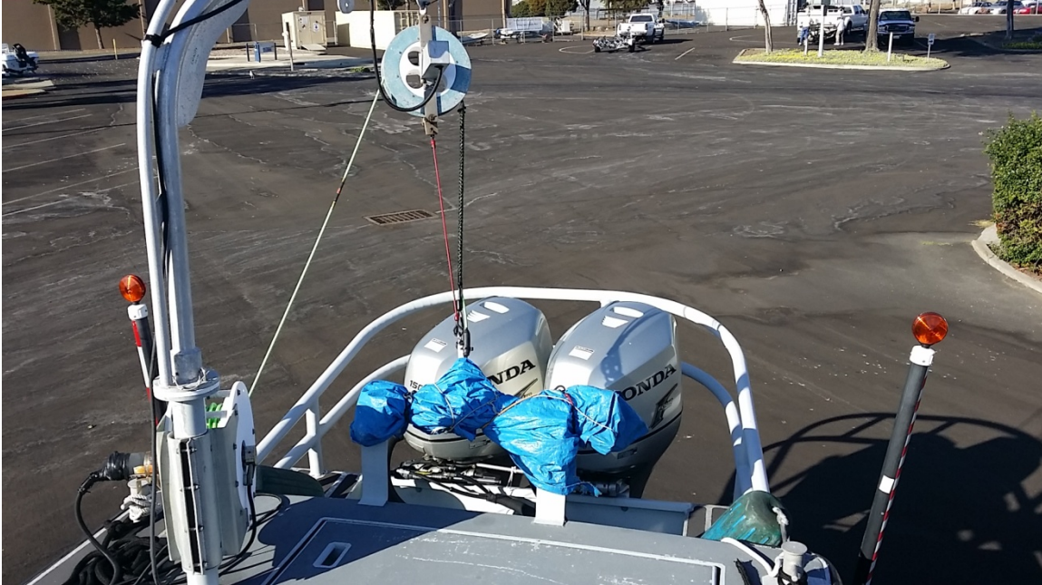
Figure 3: S3003 Edgetech 4125 SSS installation.
