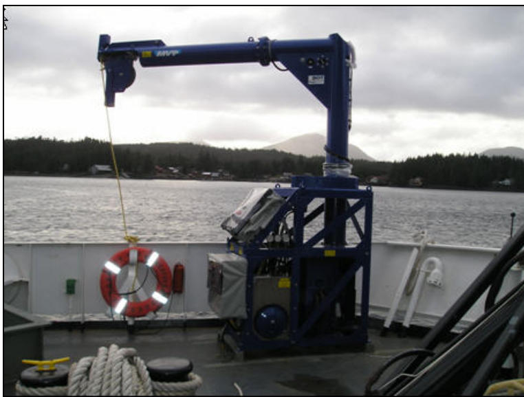
Figure 17: Fairweather's MVP200 sound velocity system
