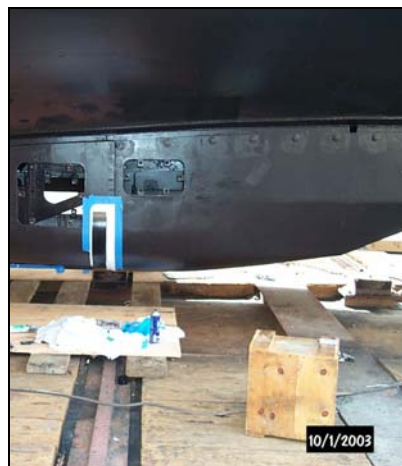
Figure 2: RESON SeaBat 8111ER MBES on Fairweather
