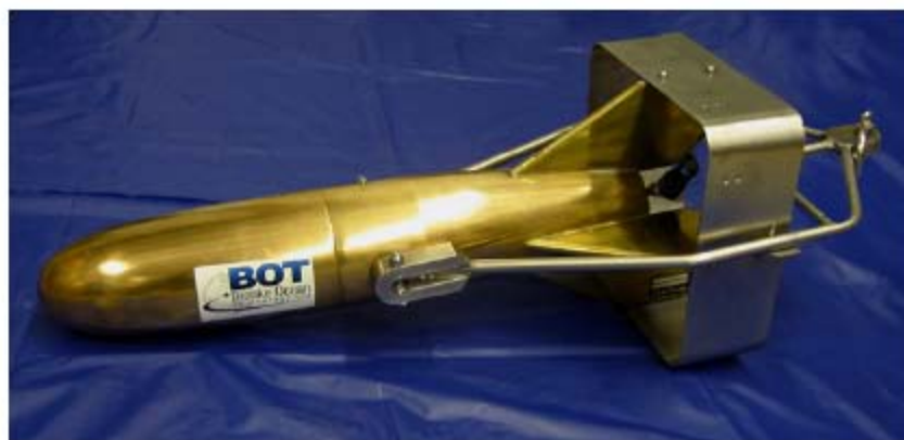
Figure 3: Single Sensor Free-Fall Fish
