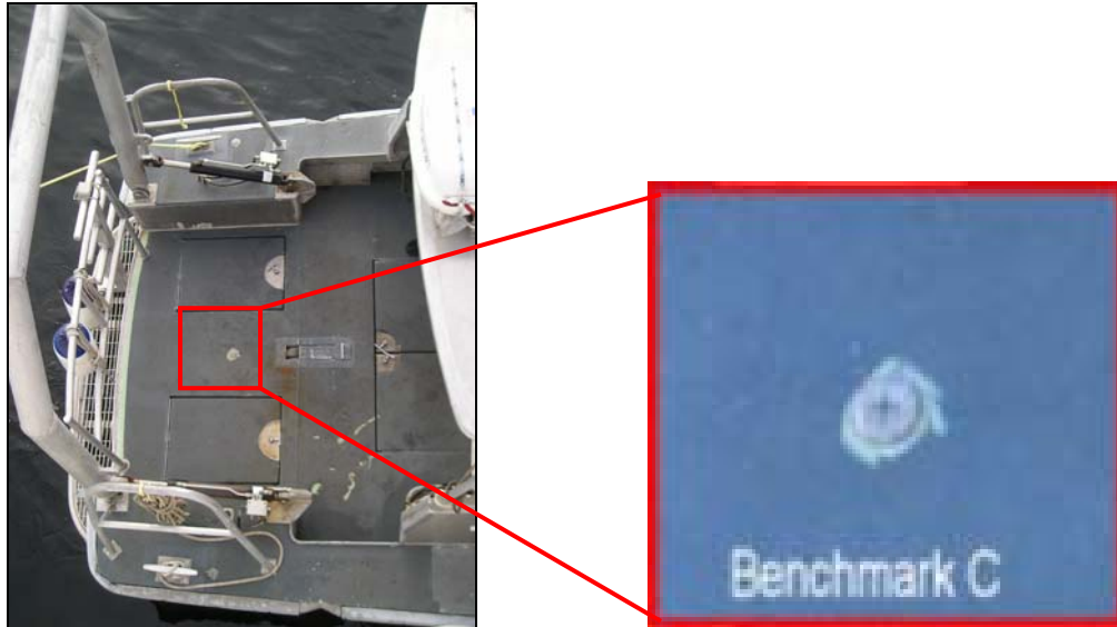
Figure 20: Permanent Control Point "Benchmark C" on launch 1018
