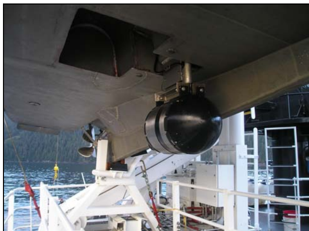
Figure 5: Launch 1010 with 8101 extended
