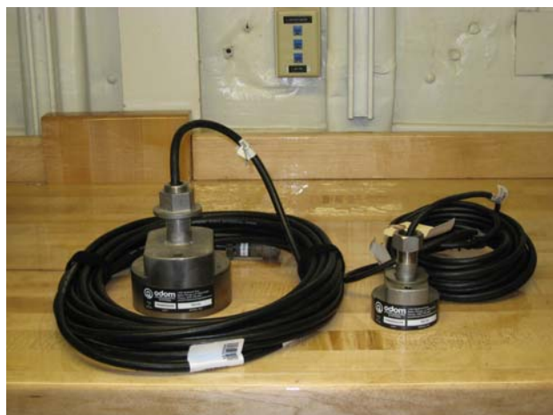
Figure 9: Four degree (left) & nine degree transducers
