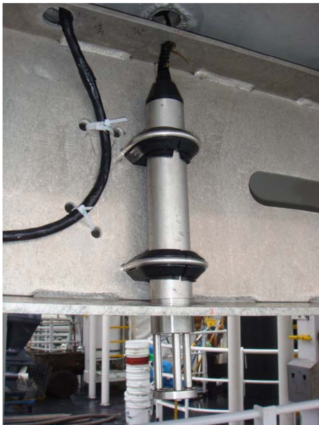
Figure 19: Fairweather 's Odom Digibar Pro mounted on Launch 1018.
