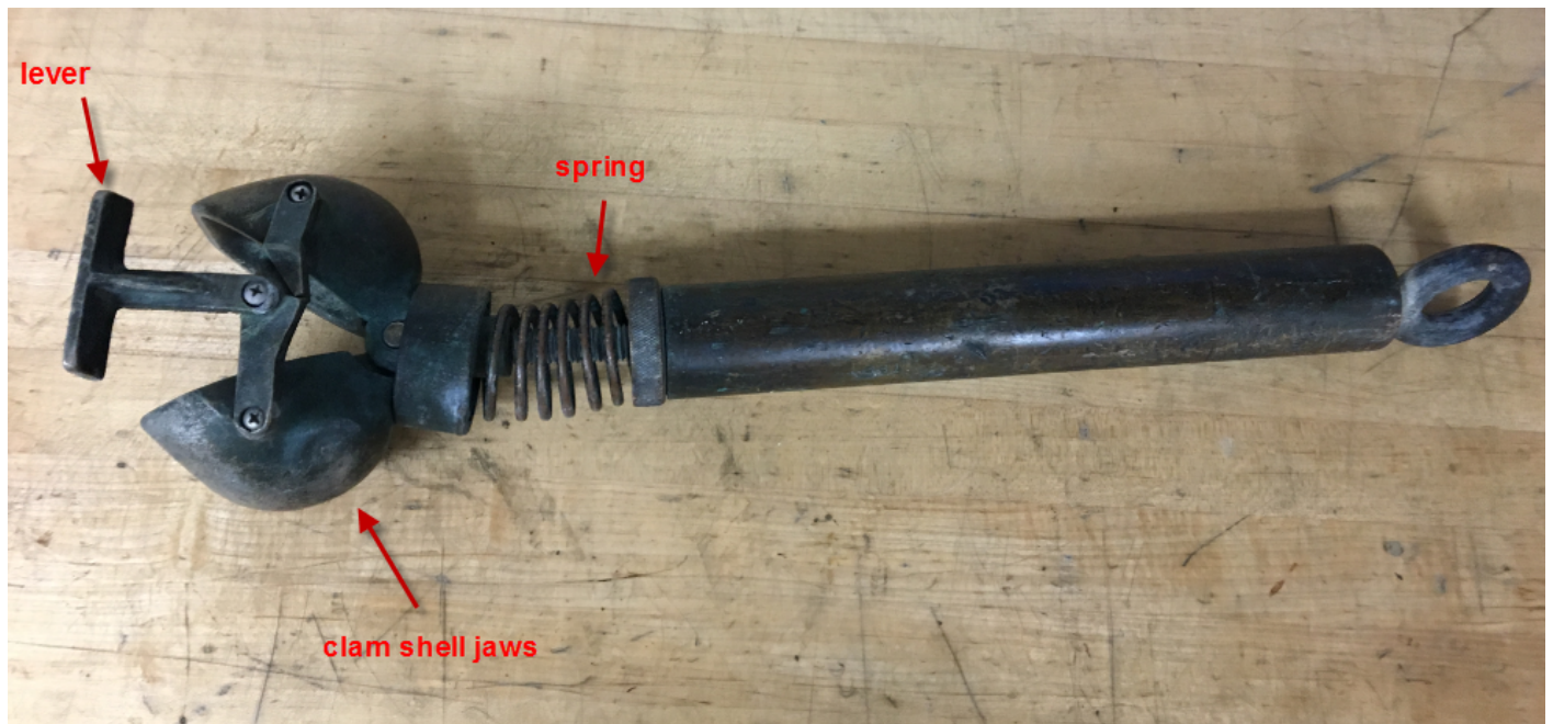
Figure 13: Mud Snapper style grab sampler used about NOAA Ship Fairweather launches.
