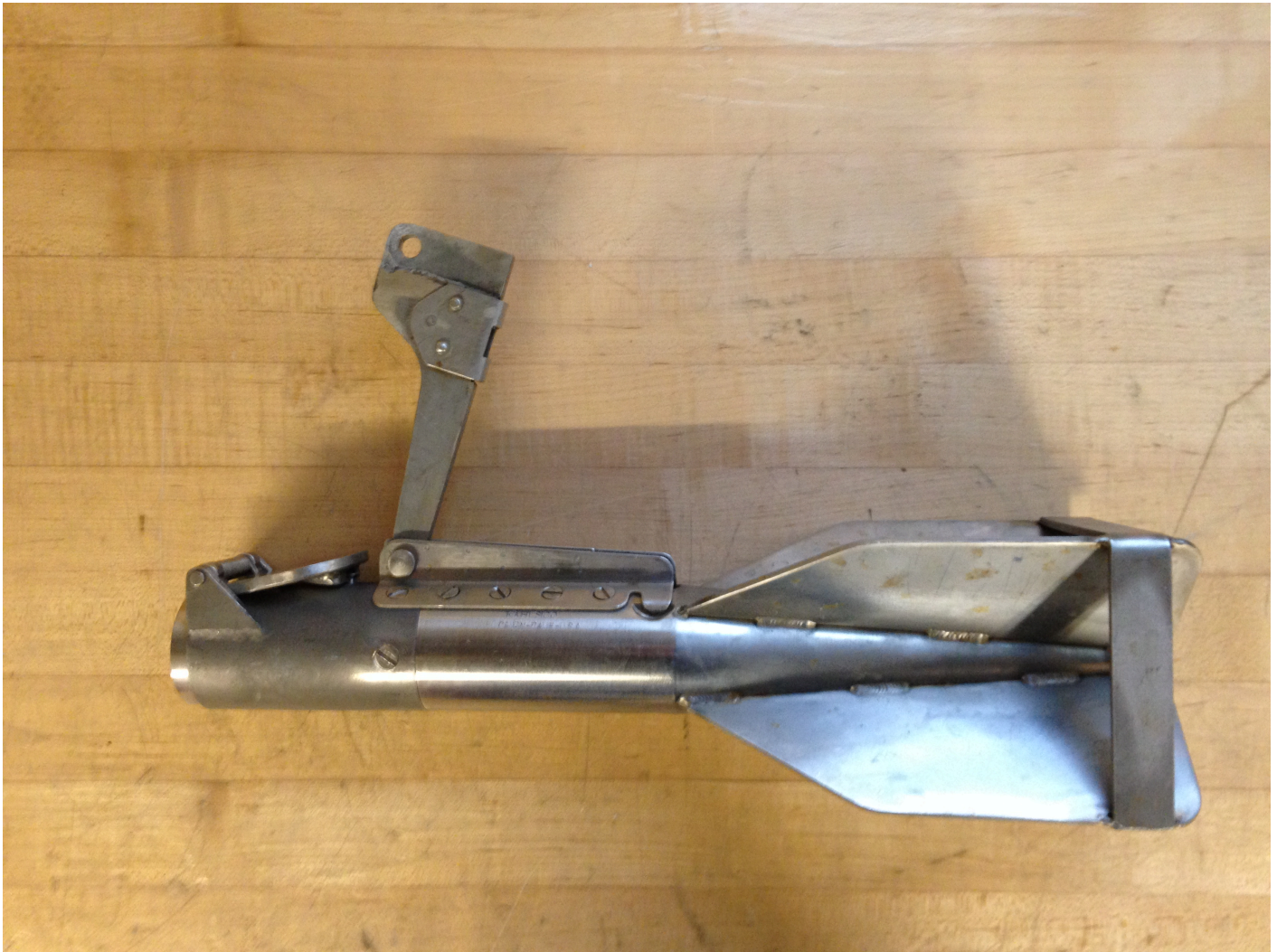
Figure 14: Torpedo style grab sampler used about NOAA Ship Fairweather launches.
