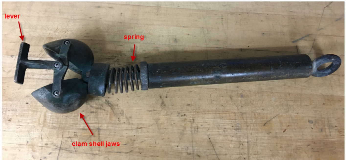
Figure 11: Mud Snapper style grab sampler used aboard NOAA Ship Fairweather launches.
