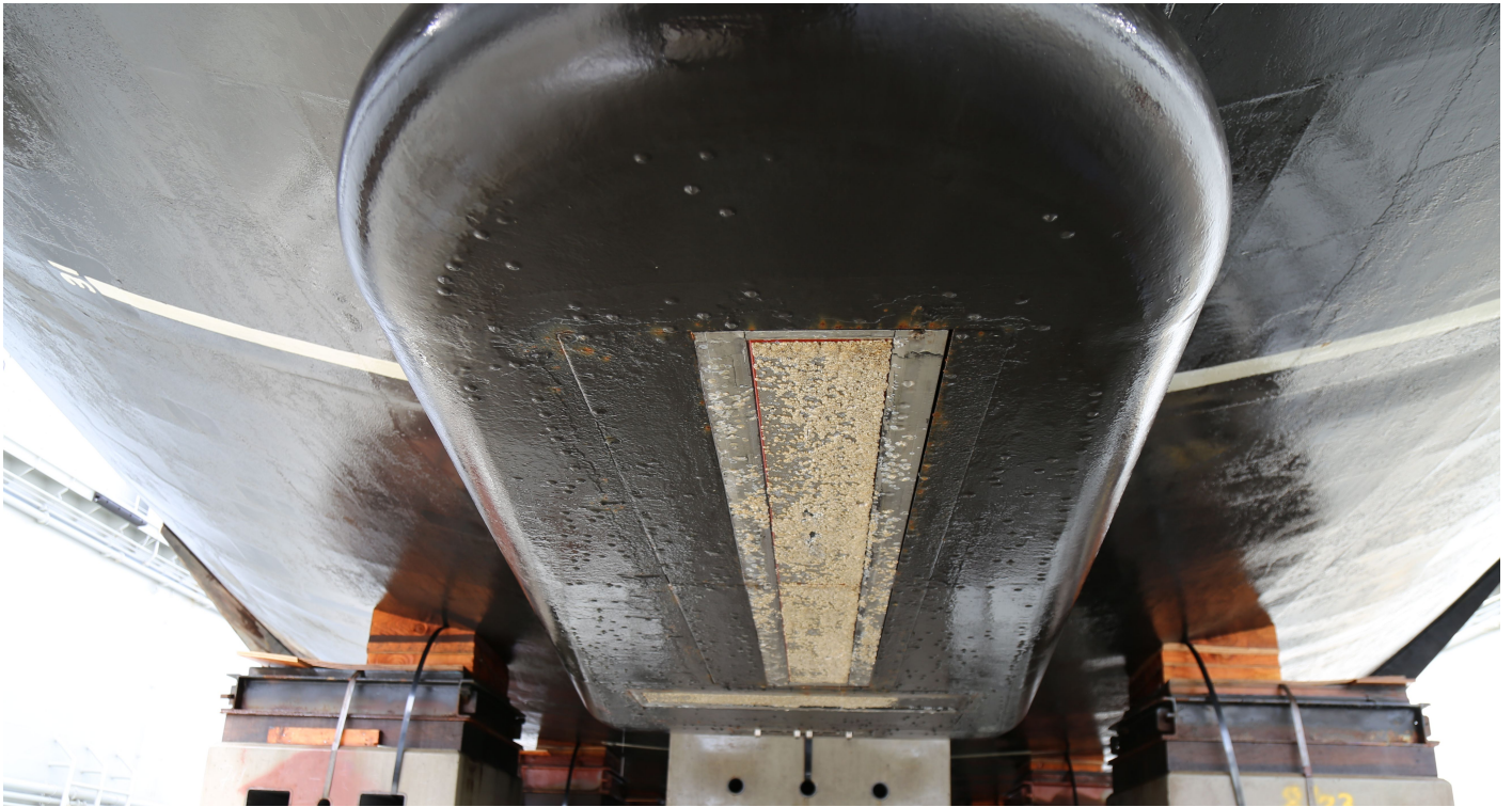
Figure 2: Kongsberg EM710 sonar transducer housing on Rainier (S221).
