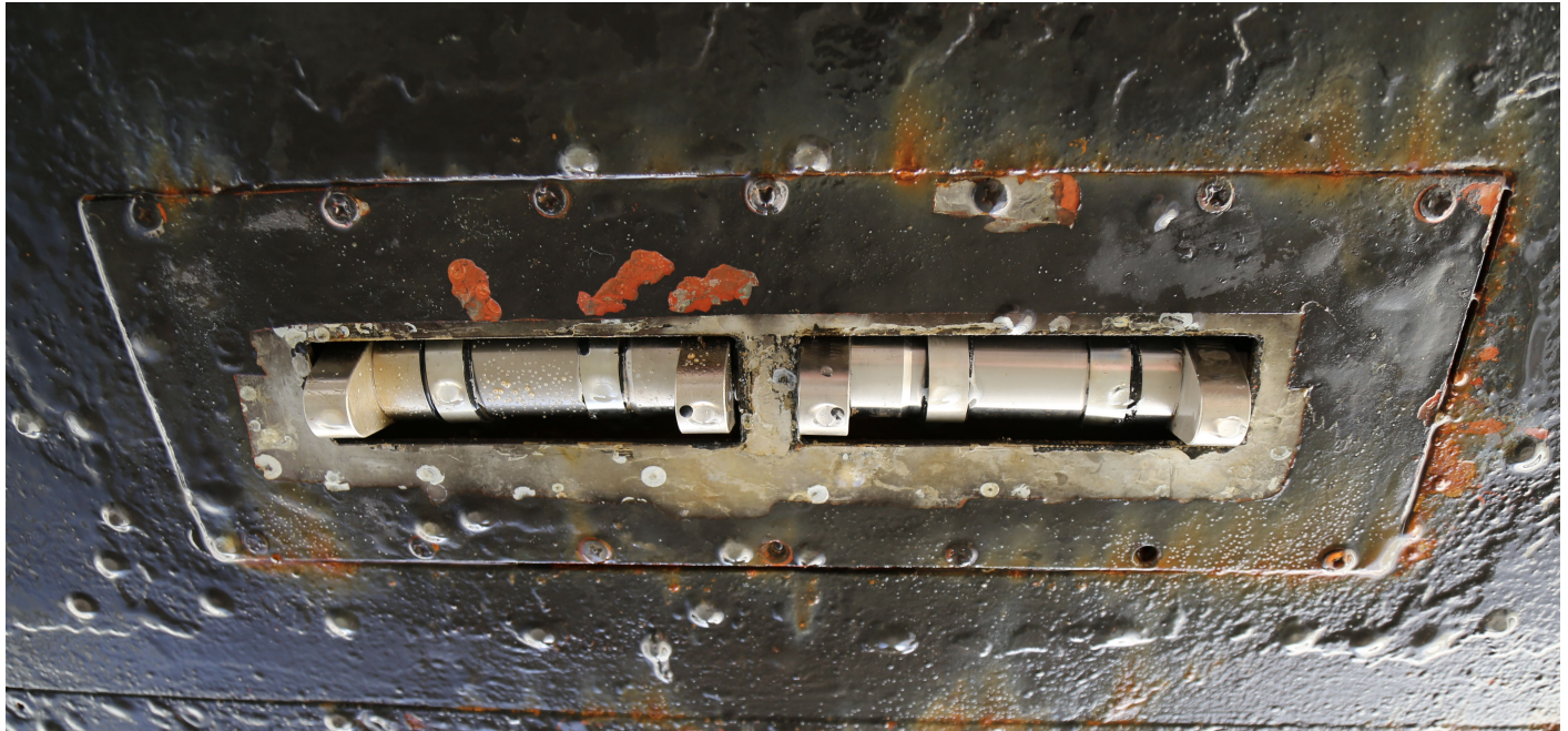
Figure 3: Dual SVP 70s mounted in Rainier's multibeam sonar transducer gondola.
