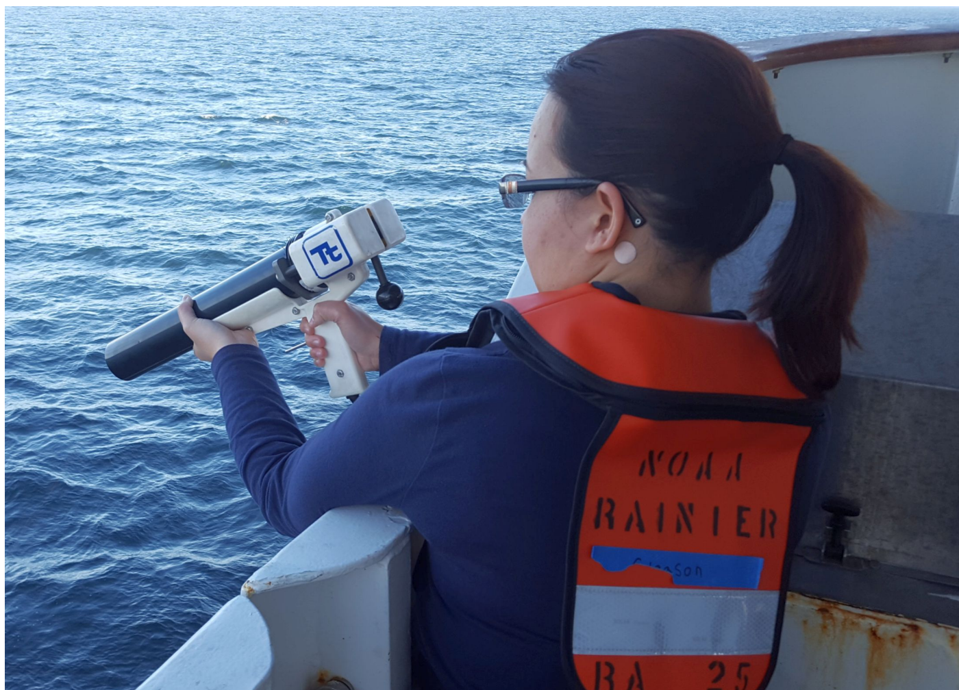
Figure 4: Deploying a XBT from the port-side bridge wing of Rainier.
