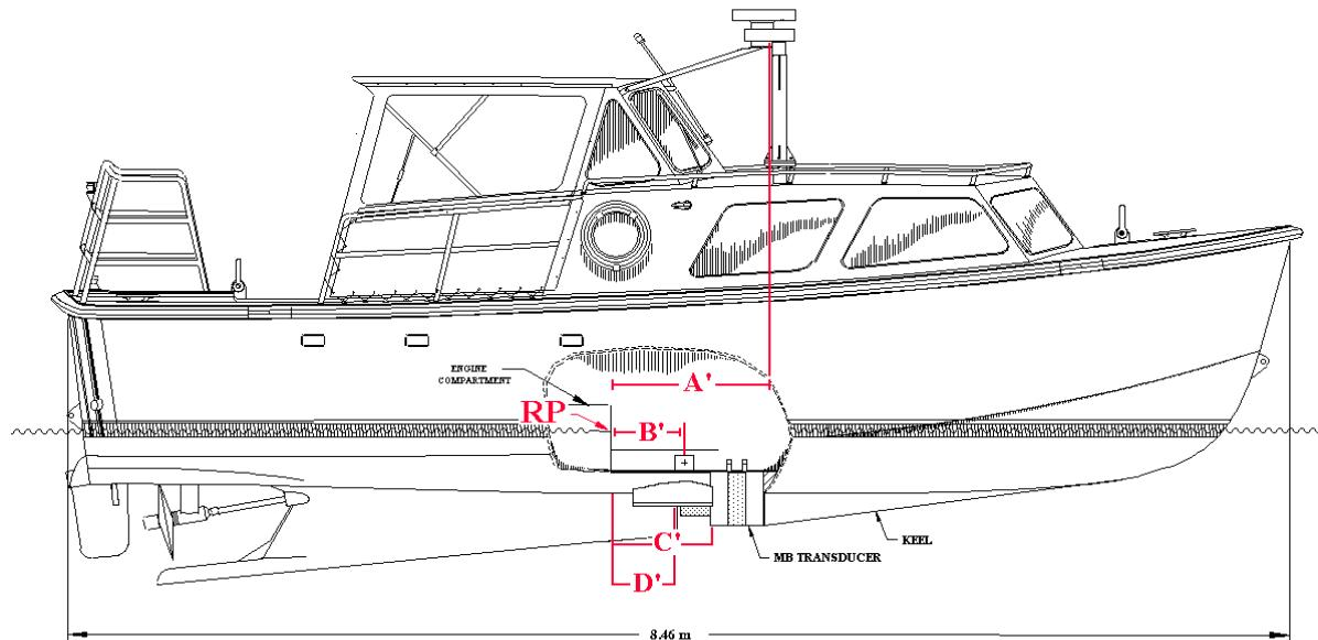
\* Assume RP at waterline & centerline of engine bulkhead
