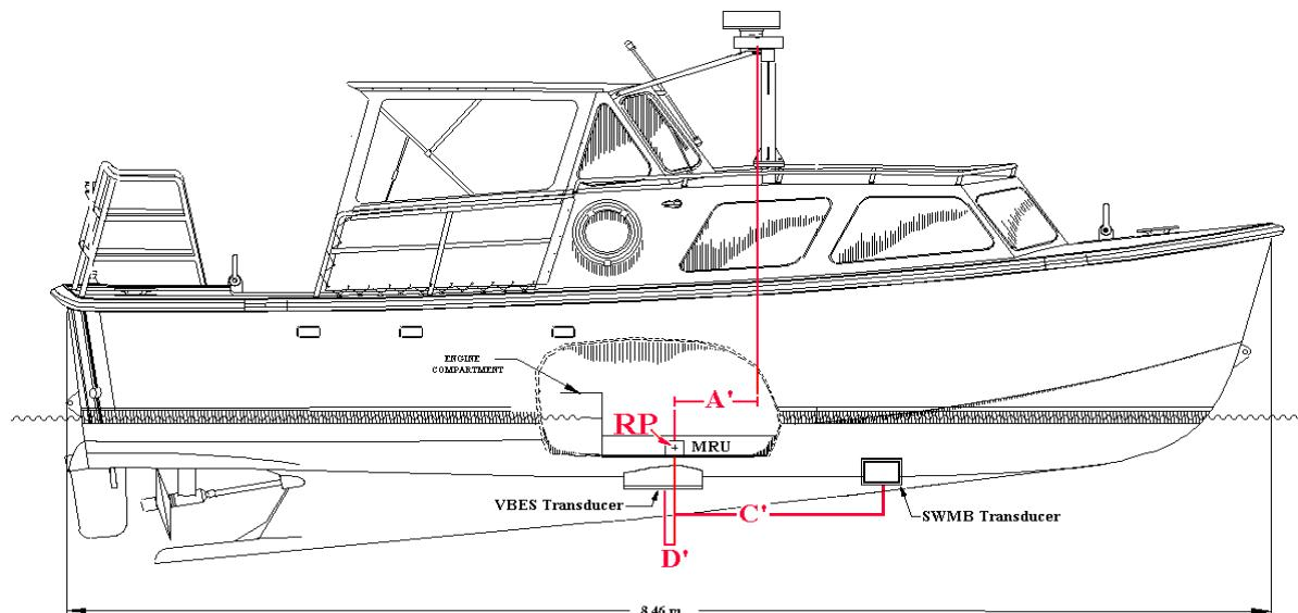
\* Assume RP at waterline & centerline of engine bulkhead
