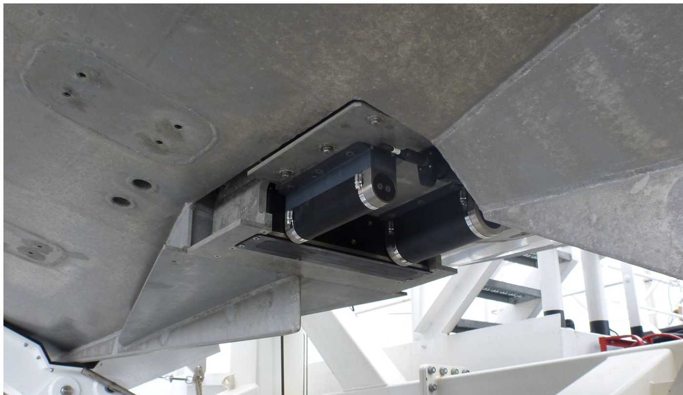
Figure 9: Reson SeaBat 7125-B mounted on survey launch 2801.
