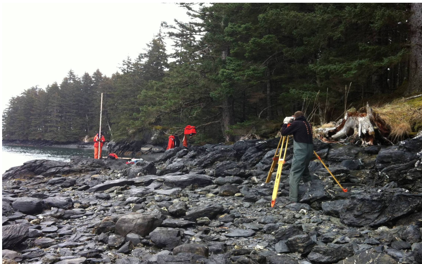
Figure 20: A Zeiss Ni2 optical level being used in the field.
