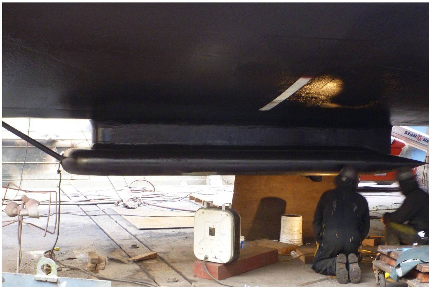
Figure 8: Kongsberg EM710 sonar transducer housing on Rainier (S221).
