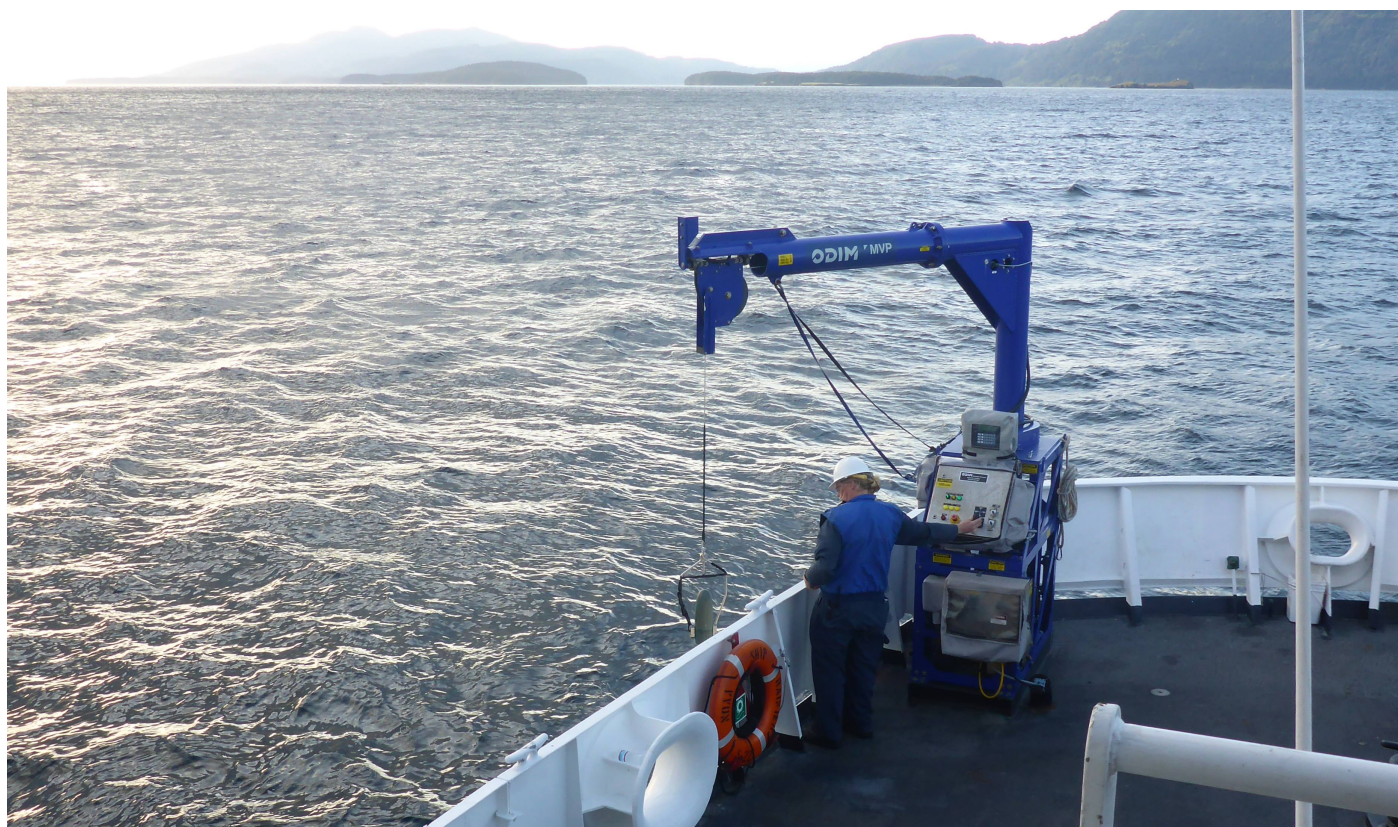
Figure 14: The ODIM Brooke Ocean MVP200 Moving Vessel Profiler being deployed from Rainier.
