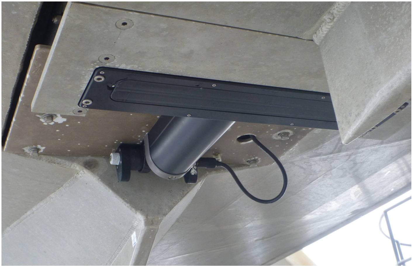
Figure 10: Reson SeaBat 7125 SV2 mounted on survey launch 2804.
