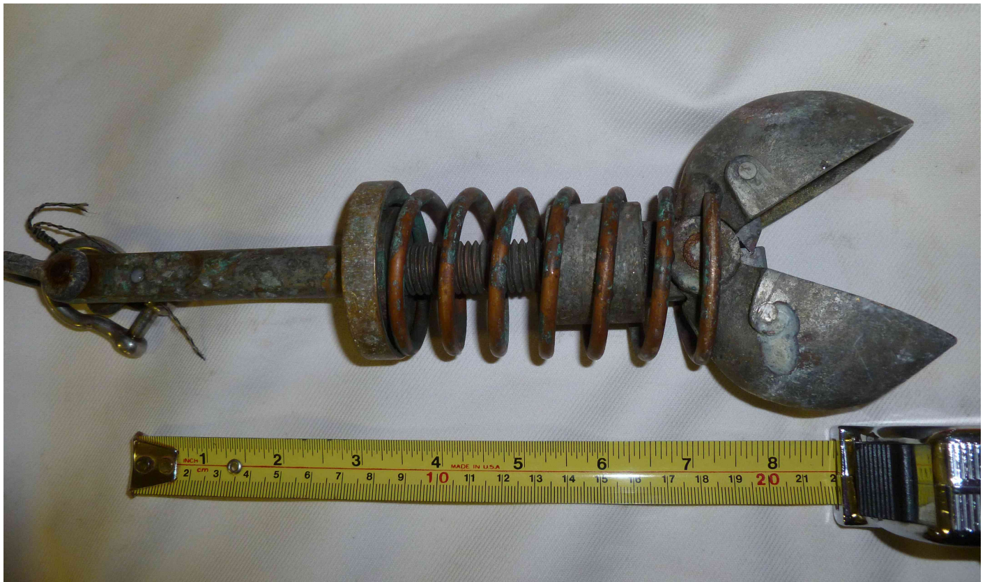
Figure 22: The “Nibbler” clam shell style bottom sampler.
