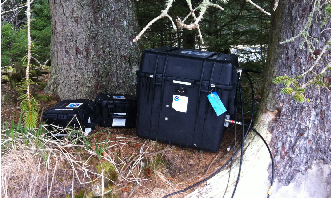
Figure 18: The Portable Tide Gauge (PTG) system, 9210B data collection platform.
