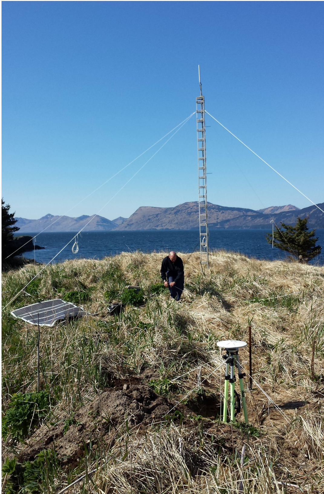
Figure 28: A Rainier base station installed in Kupreanof Strait, Kodiak Island, Alaska. Note the UHF antenna mounted on top of the 20 foot tower for extended range.
