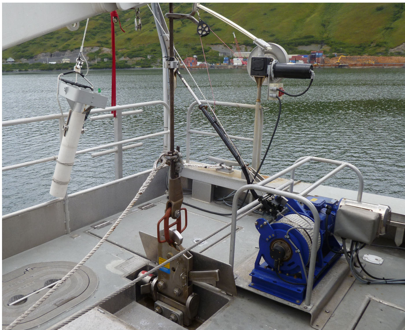
Figure 16: The ODIM Brooke Ocean MVP30 Moving Vessel Profiler as mounted aboard 2804.
