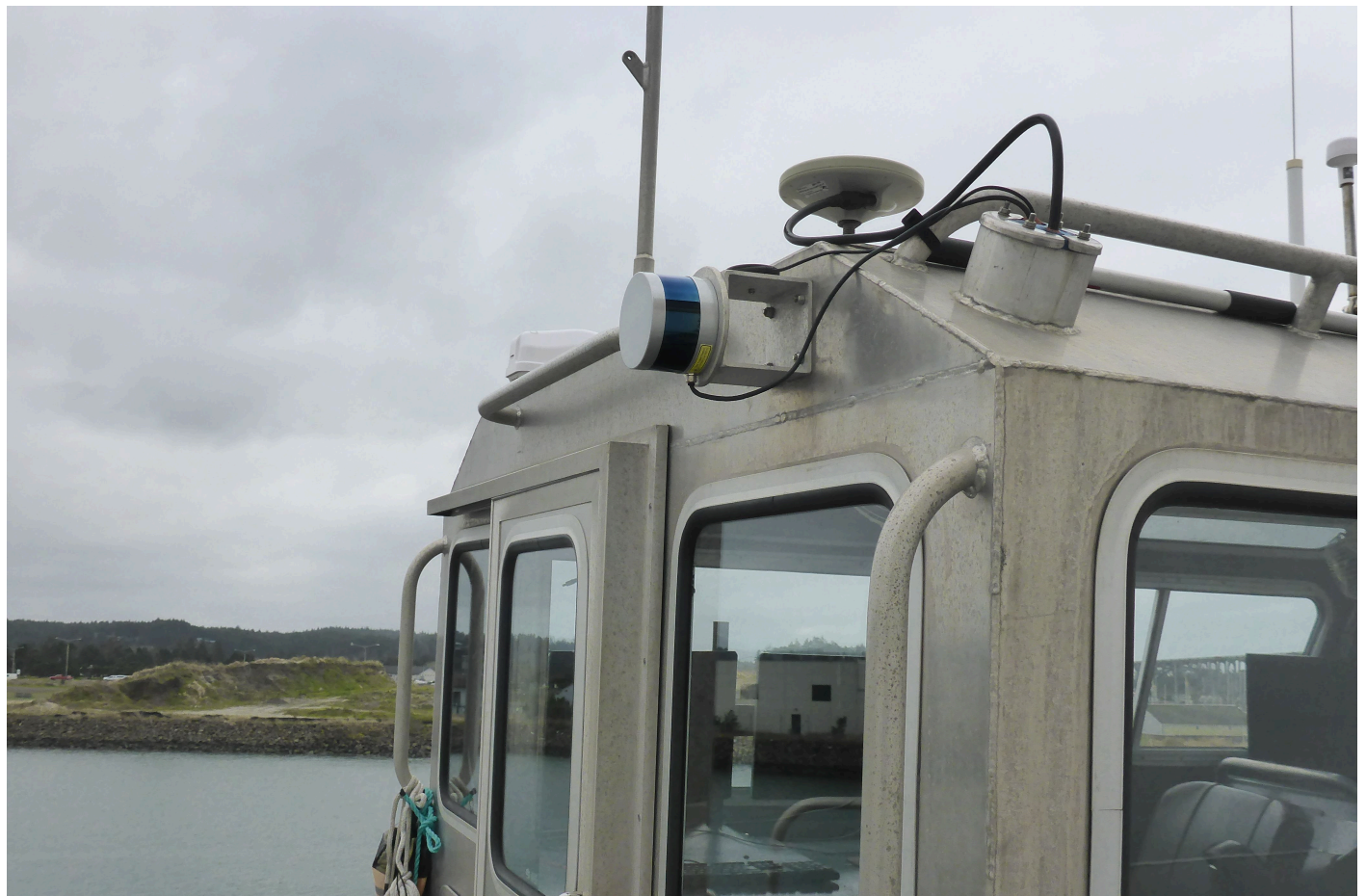
Figure 11: The Velodyne VLP-16 as mounted on 2701.
