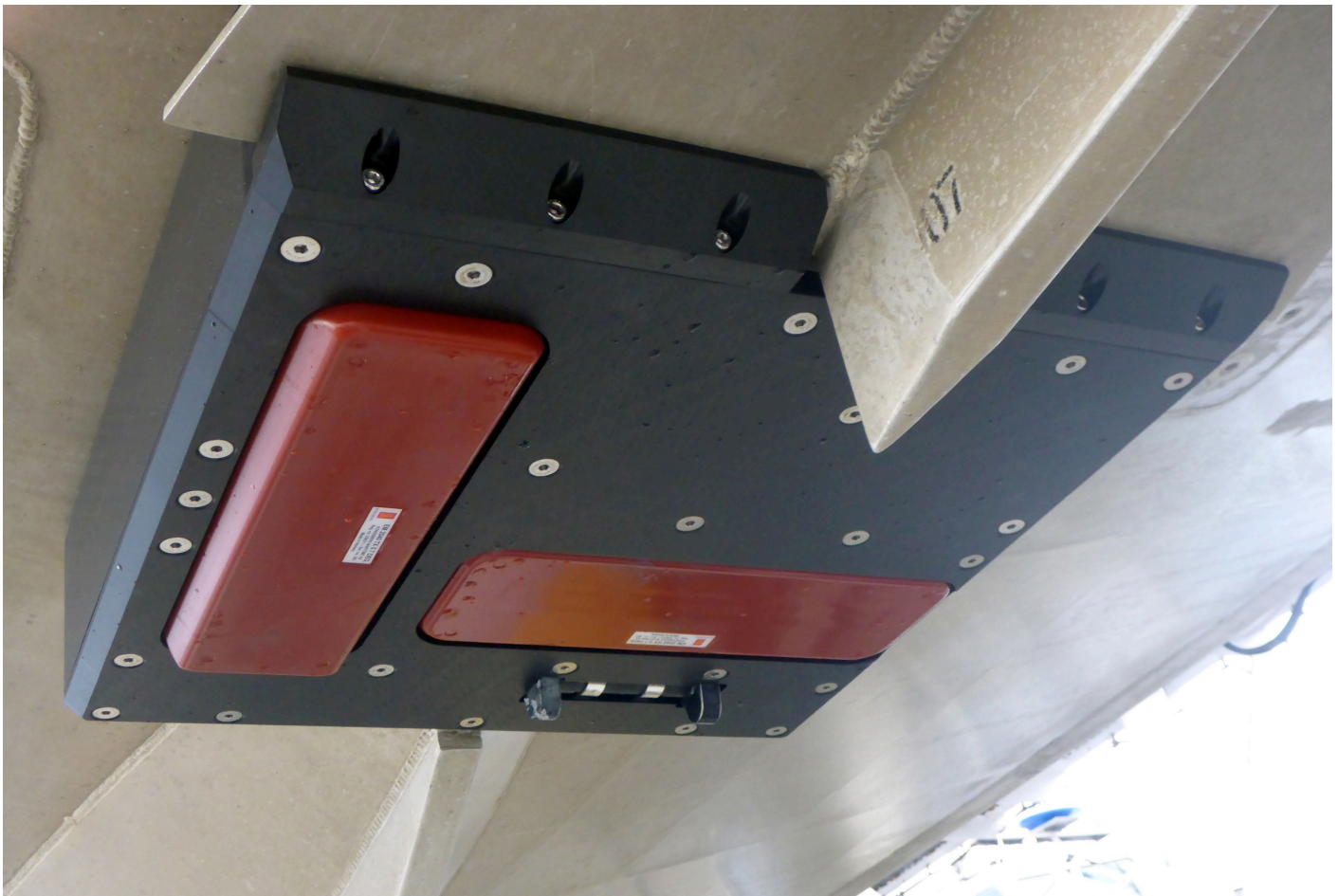
Figure 9: The Kongsberg EM2040-07 mounted on survey launch 2803.
