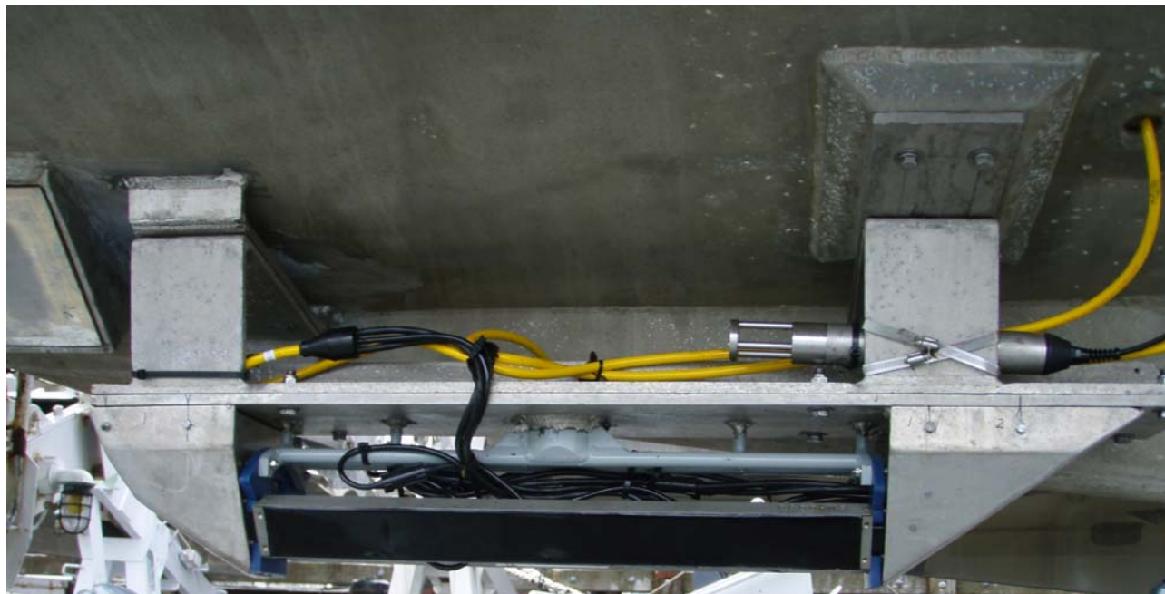
Figure 1. Teledyne Benthos C3D-LPD Phase Differencing Sonar, as installed on Launch 1015 (RA-6)
