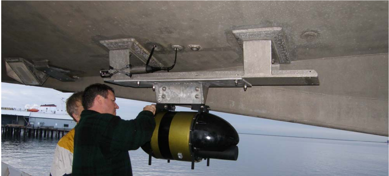
Figure 1 Reson 8101 sonar head, as installed on Launch 1015 (RA-6)
