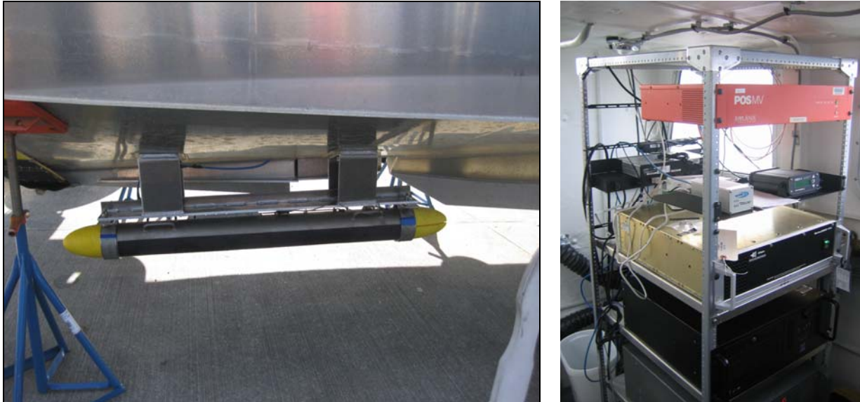
Figure 6: Hull-Mounted Klein 5000 Side Scan Sonar on Fairweather Launch with TPU
