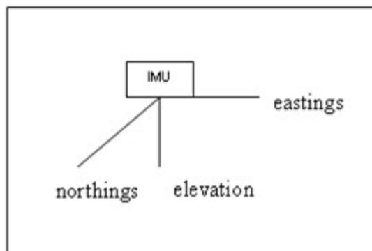
Bottom Center of IMU is origin of Westlake Coordinate System
