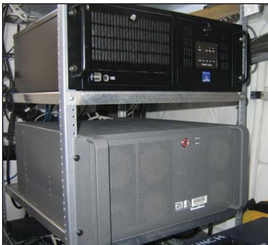
Figure 1: Reson 7125 SV topside processor
