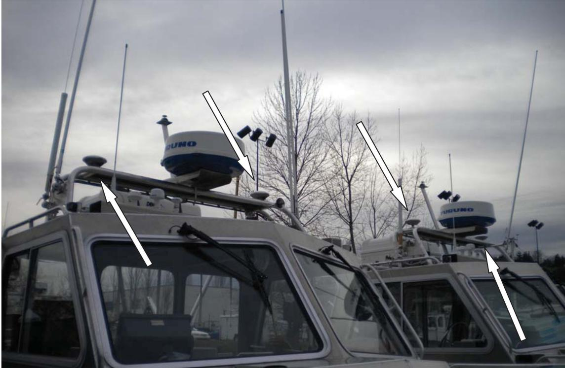
**Figure 10: POS GNSS Antennas**
