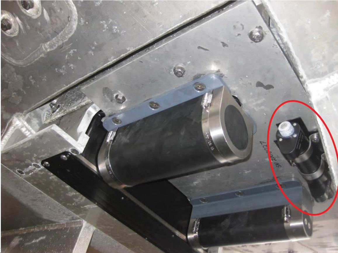
**Figure 16: SVP 71 sound speed unit (right) and a Reson 7125**
