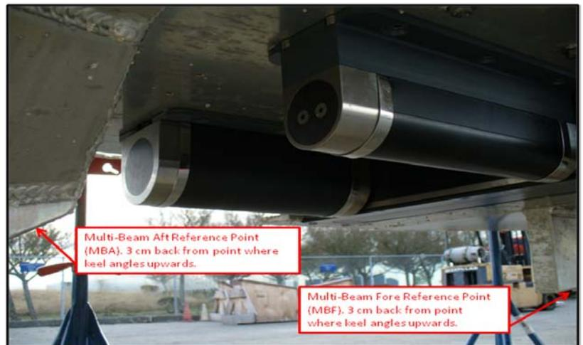
A point on the Multi-Beam transducer (MB) was measured directly this survey. The measured point was at the center of the bottom of the transducer. No mark was left to indicate the measured point.
