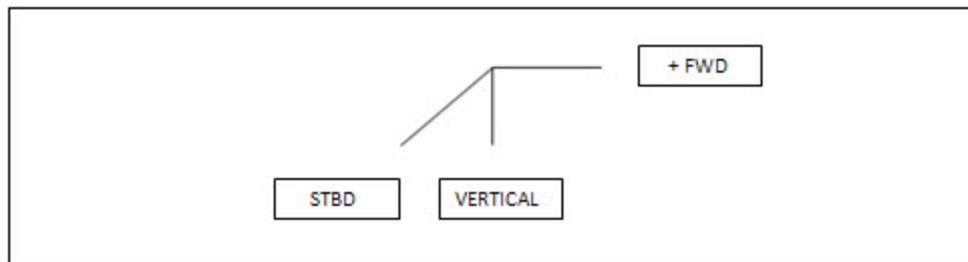
Top Center of IMU is origin of Hypack Coordinate System
