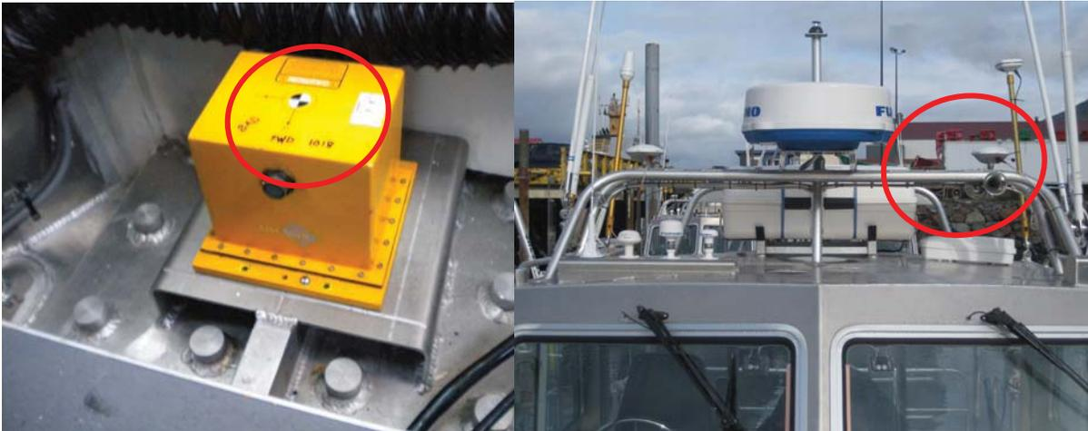
**Figure 17: Vessel Reference Point (Top of POS MV IMU) & Primary GNSS Antenna (port side).**
