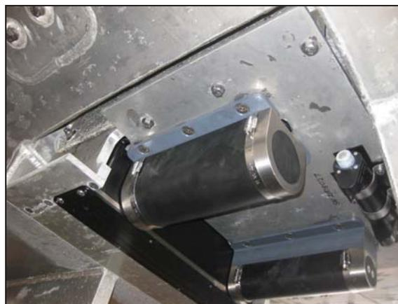
Figure 6: Reson 7125 SV transducer arrays
