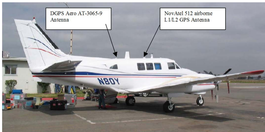
Figure B17 - NovAtel GPS Antenna and Aero DGPS Antenna locations
