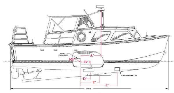
\* Assume RP at waterline & centerline of engine bulkhead
