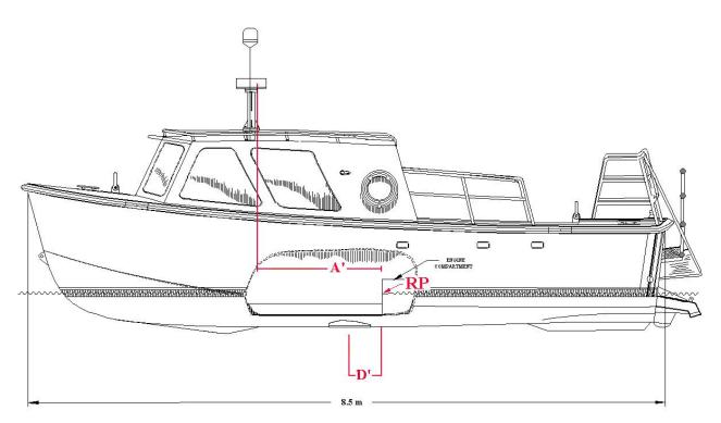
\* Assume RP at waterline & centerline of engine bulkhead
