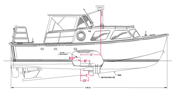
\* Assume RP at waterline & centerline of engine bulkhead
