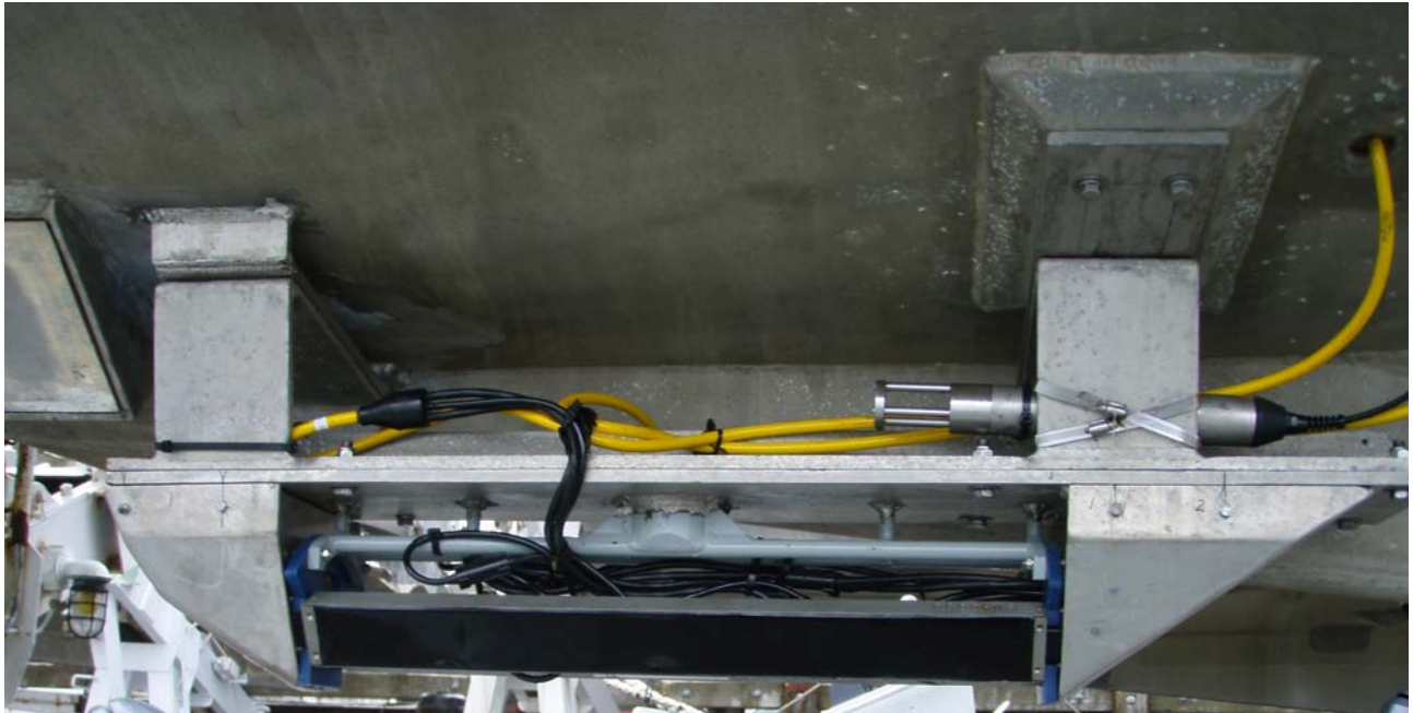
Figure 1. Teledyne Benthos C3D-LPD Phase Differencing Sonar, as installed on Launch 1015 (RA-6)
