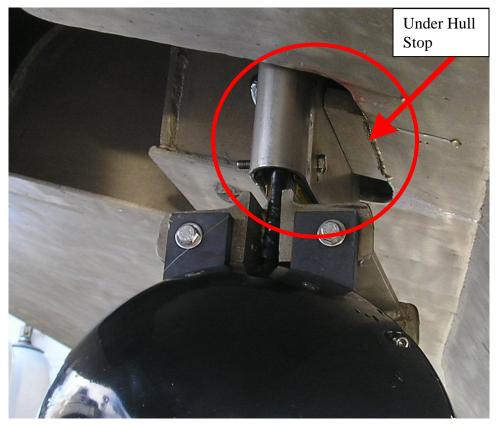
Figure 6: Launch 1010 swing arm mount against hull stop.
