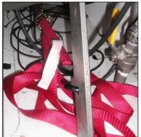
Figure 13: Rachet strap attachment point to arm.
