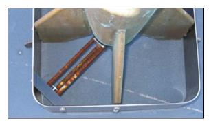
Figure 8: Rusted MVP 200 sensor.
