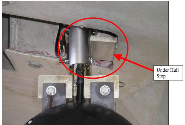
Figure 12: Launch 1010 swing arm mount against hull stop.
