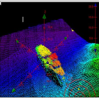
Figure 2: Heading and Pitch patch test site for Launch 1010.
