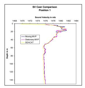
Figure 4: Sound velocity profiles from Position 1.
