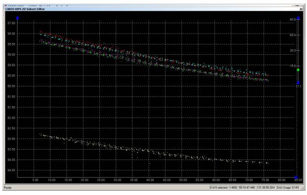
Figure 2: Across-track view of Roll patch lines from DN 071 and DN 072, with a vertical offset of approximately 4.7 m between days
