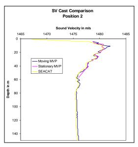
Figure 5: Sound velocity profiles from Position 2.
