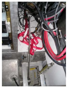
Figure 9: The deployment lever arm, set pin and ratcheting tie-down strap. The pin was eventually removed to allow the arm to reach the under hull stop.
