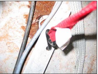
Figure 14: Rachet strap attachment point to hull.
