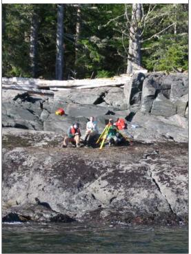
Figure 7: Settlement and Squat shore team using optical level.
