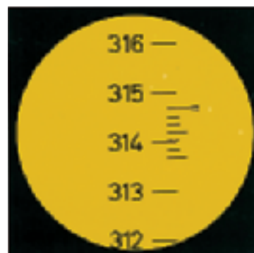
NAK2 circle reading (360°) 314°42'
