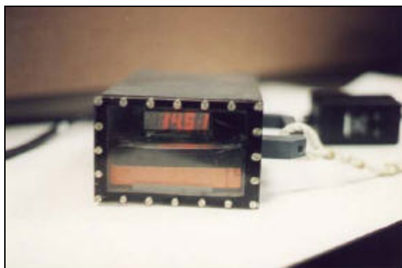
Figure 11: Diver's least depth gauge
