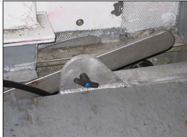
Figure 8: Stainless steel pin locked in to with transducer up
