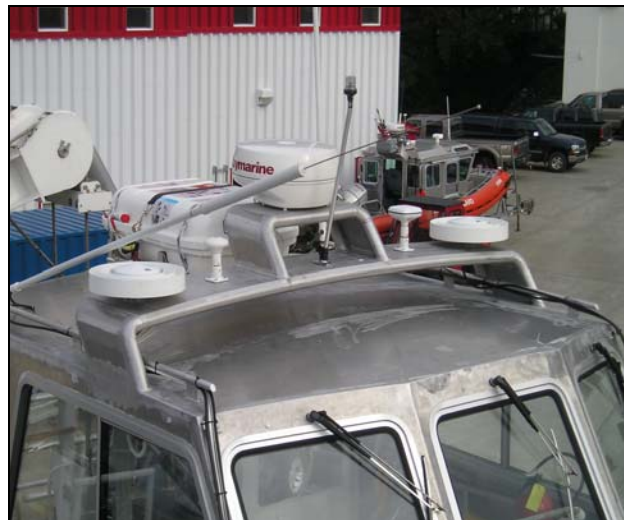
Figure 4: POS/MV antennas mounted on 1010 (side view)
