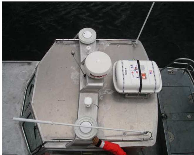
Figure 3: POS/MV antennas mounted on 1018 (top view)
