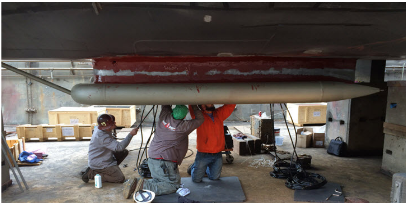
Figure 6: EM 710 gondola during transducer installation
