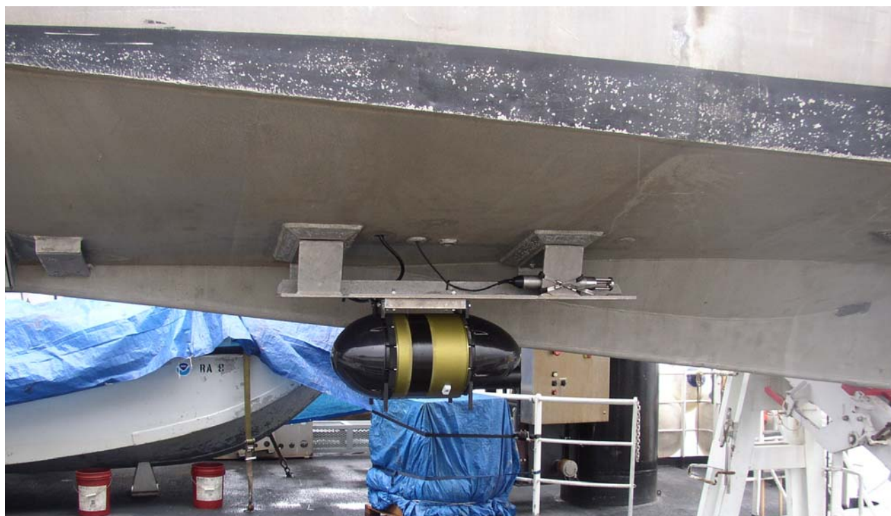
Figure 1 Reson 8101 sonar head, as installed on Launch 1015 (RA-6)
