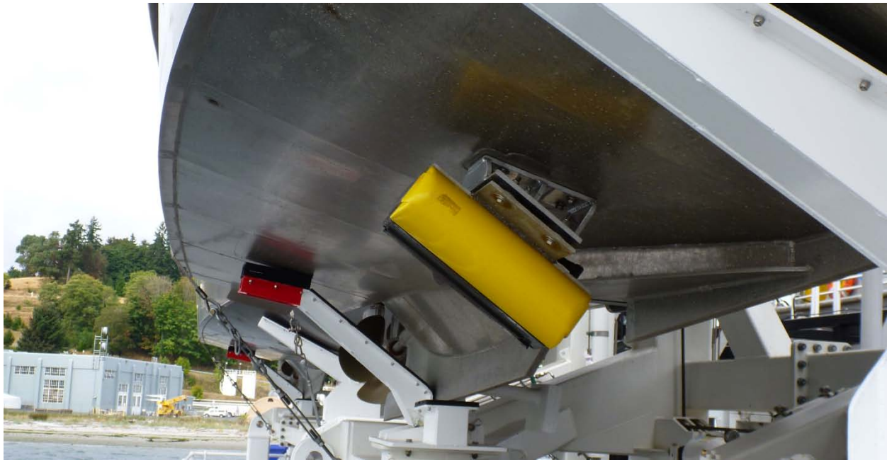
Figure 1 Reson Seabat 8125 mounted on survey launch 2803
