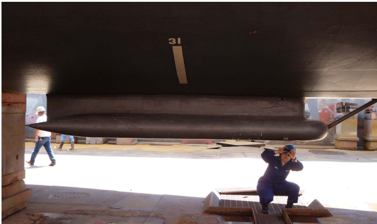
Figure 2 Kongsberg EM 710 sonar transducer housing on Rainier (S221)
