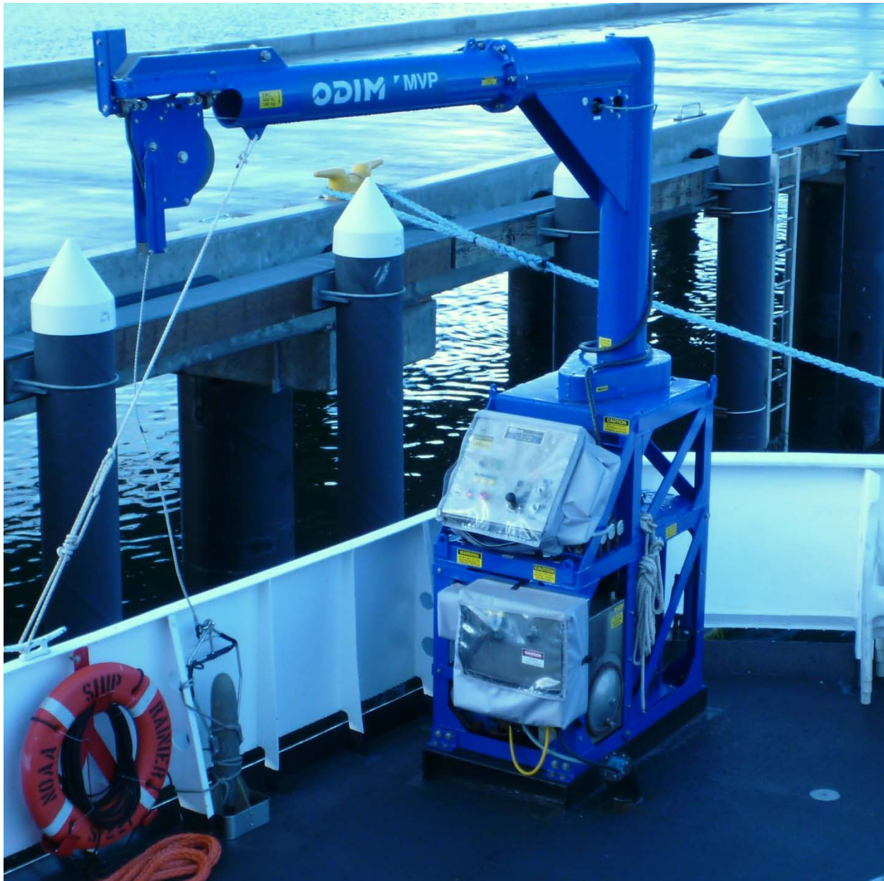
Figure 4 The ODIM Brooke Ocean MVP200 Moving Vessel Profiler mounted aboard Rainier
