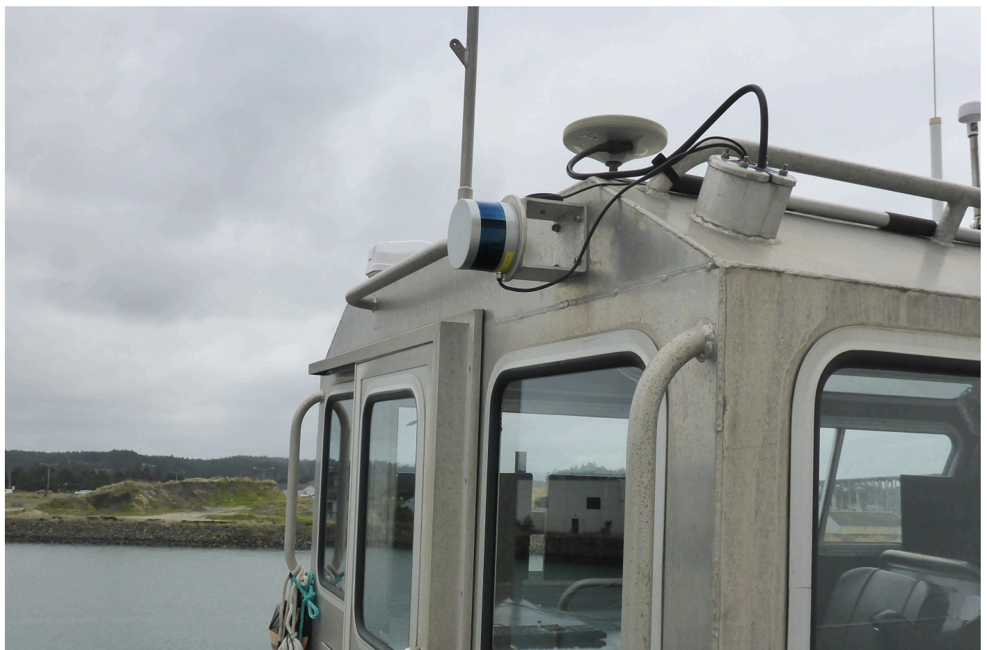
Figure 11: The Velodyne VLP-16 as mounted on 2701.
