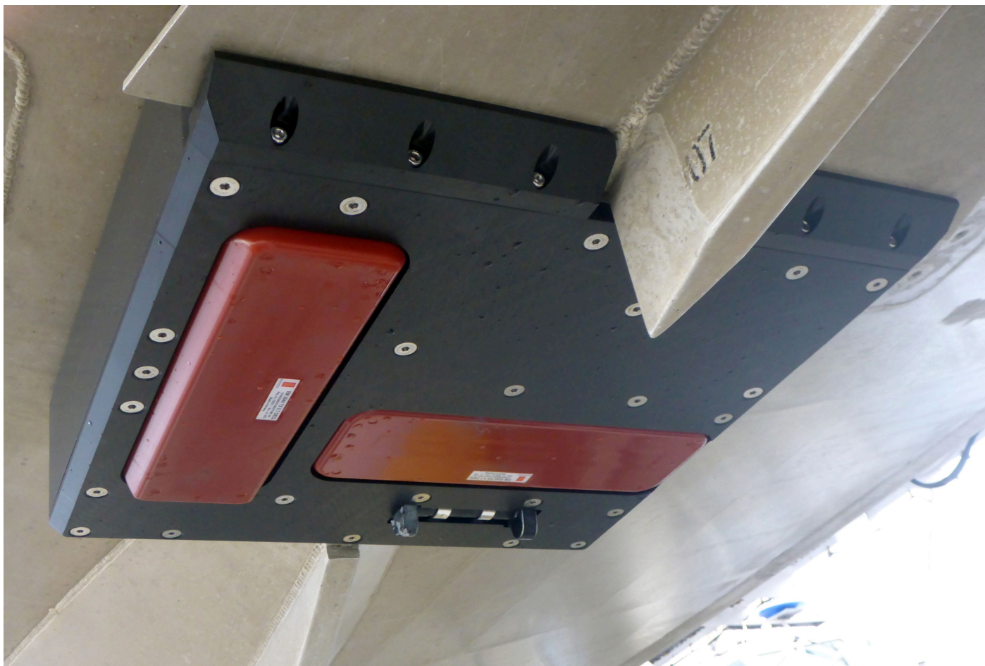
Figure 9: The Kongsberg EM2040-07 mounted on survey launch 2803.
