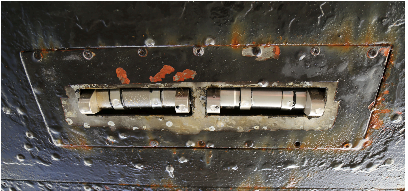
Figure 15: Dual SVP 70s mounted in Rainier's multibeam sonar transducer gondola.
