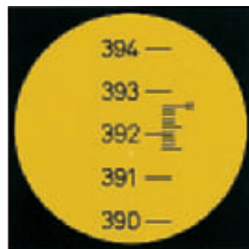
NAK2 circle reading (400 gon) 392.66 gon
