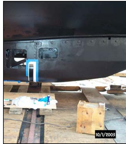
Figure 2: RESON SeaBat 8111ER MBES on Fairweather
