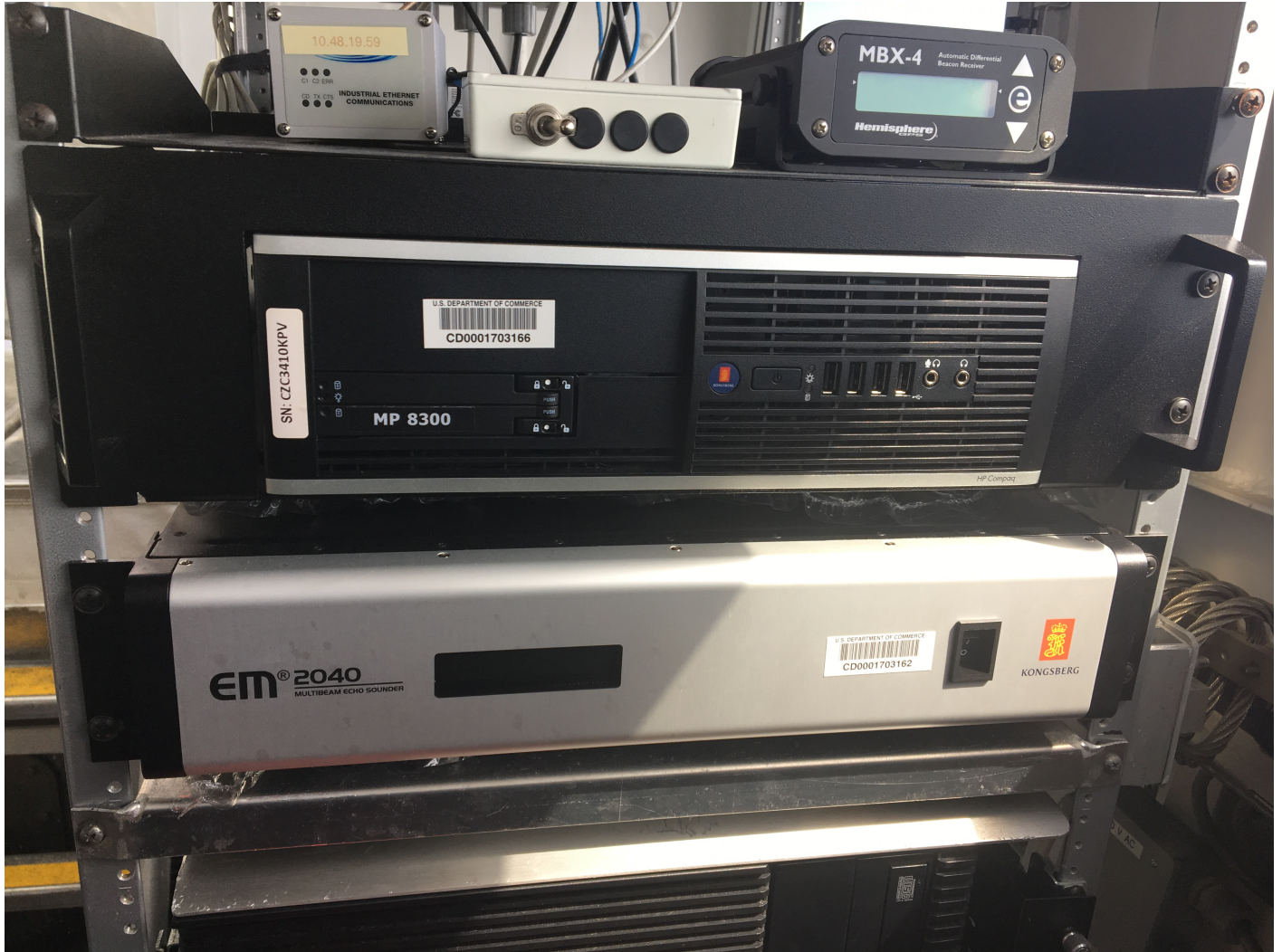
Figure 11: Kongsberg EM 2040 topside processing unit
