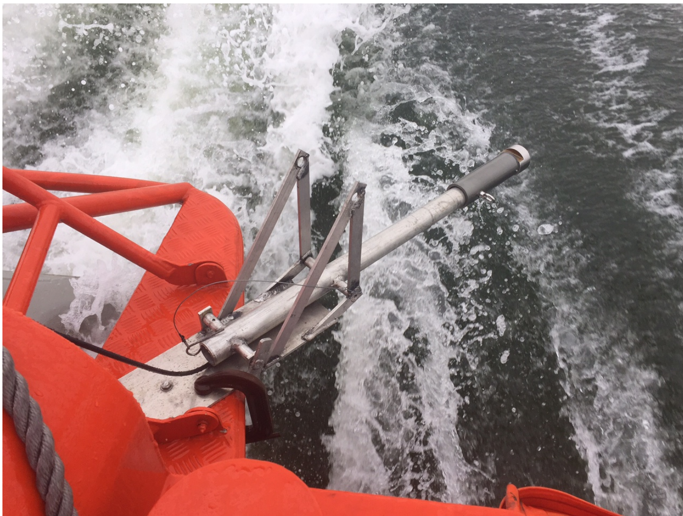
Figure 14: CEEPulse on a pole mount attached to FA 2303
