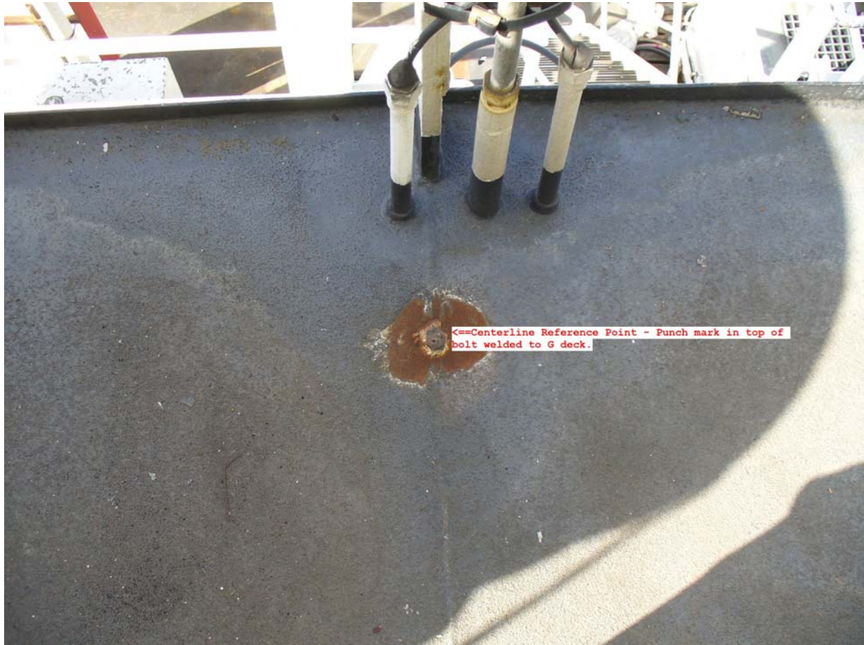
CENTERLINE REFERENCE POINT ON G DECK
