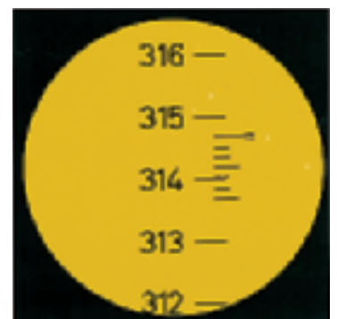
NAK2 circle reading (360°) 314°42'
