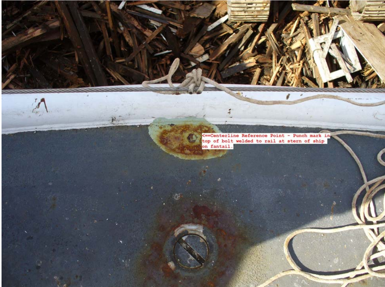
CENTERLINE STERN REFERENCE POINT
