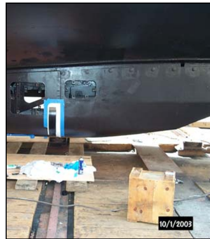
Figure 2: RESON SeaBat 8111ER MBES on Fairweather
