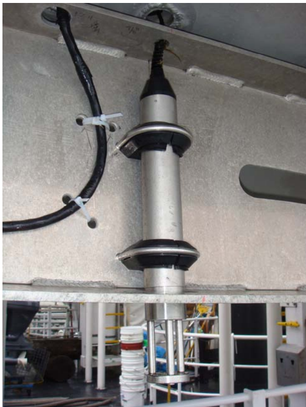
Figure 19: Fairweather's Odom Digibar Pro mounted on Launch 1018.
