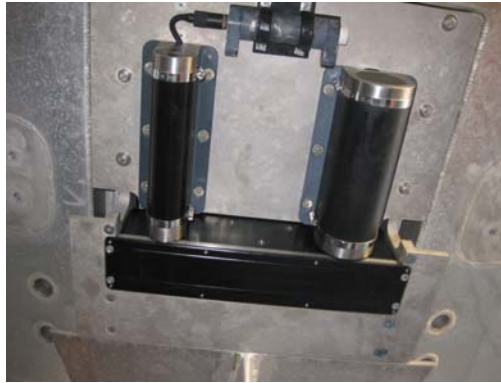
Figure 21: SVP 71 sound speed unit (top) and a RESON 7125
