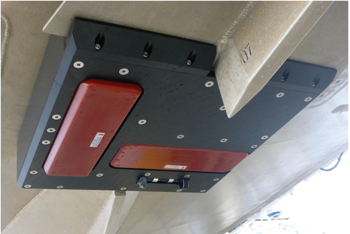
Figure 9: The Kongsberg EM2040-07 mounted on survey launch 2803.
