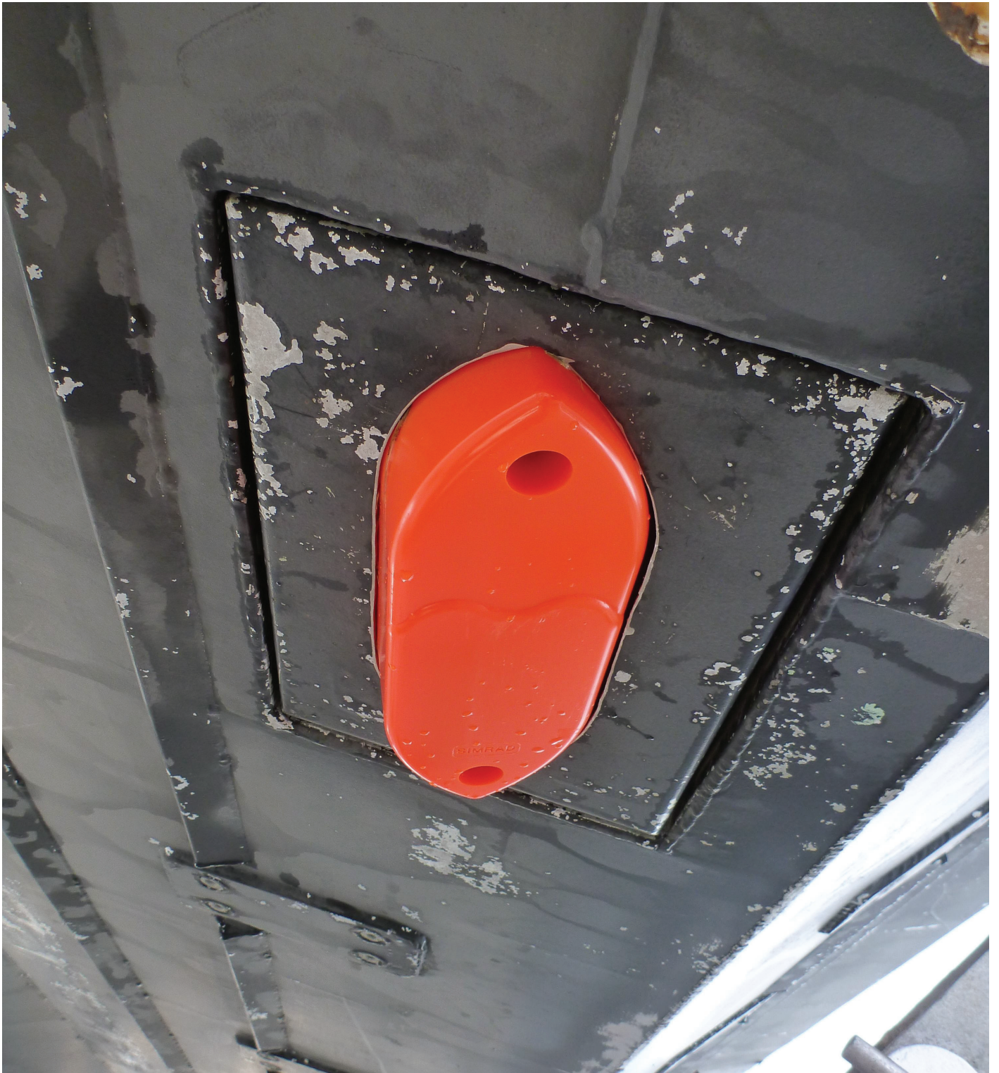
Figure 10: The Simrad 50/200 Combi D transducer as mounted on 2701 for the Teledyne Odom Hydrographic Echotrac CV200 hydrographic echo sounder.
