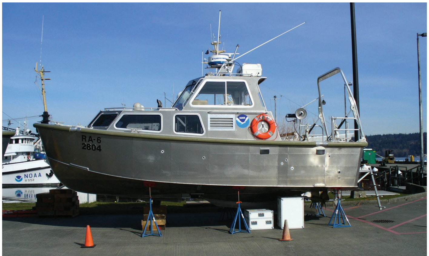
Figure 6: Rainier survey launch RA6 (2804) on blocks for her NGS offsets survey at the NOAA Western Regional Center, Sand Point, Washington.
