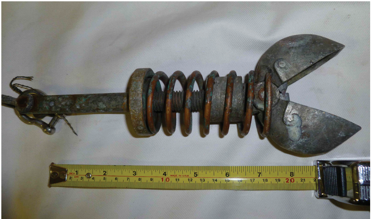
Figure 18: The “Nibbler”, a foot-trip clam shell style bottom sampler.
