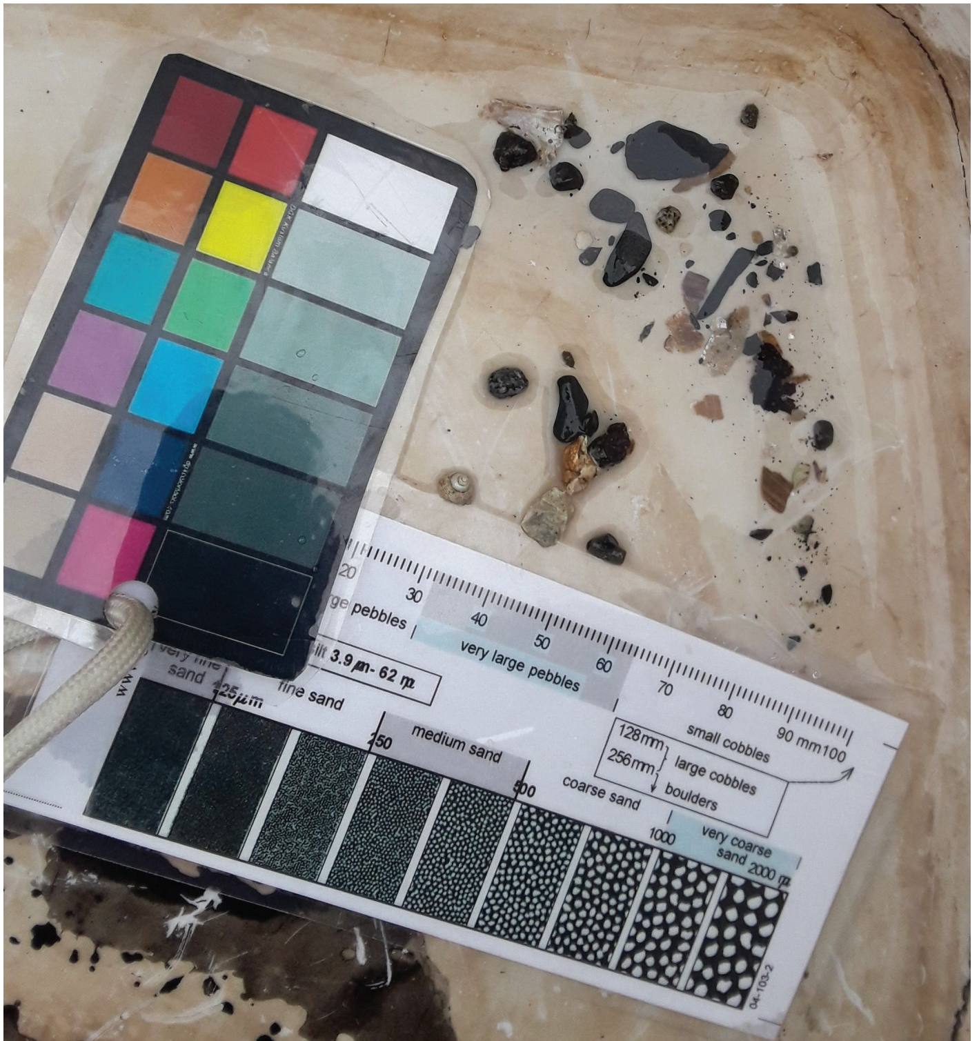
Figure 22: Bottom sample analysis using laminated cards with both color and size to classify a sediment sample
