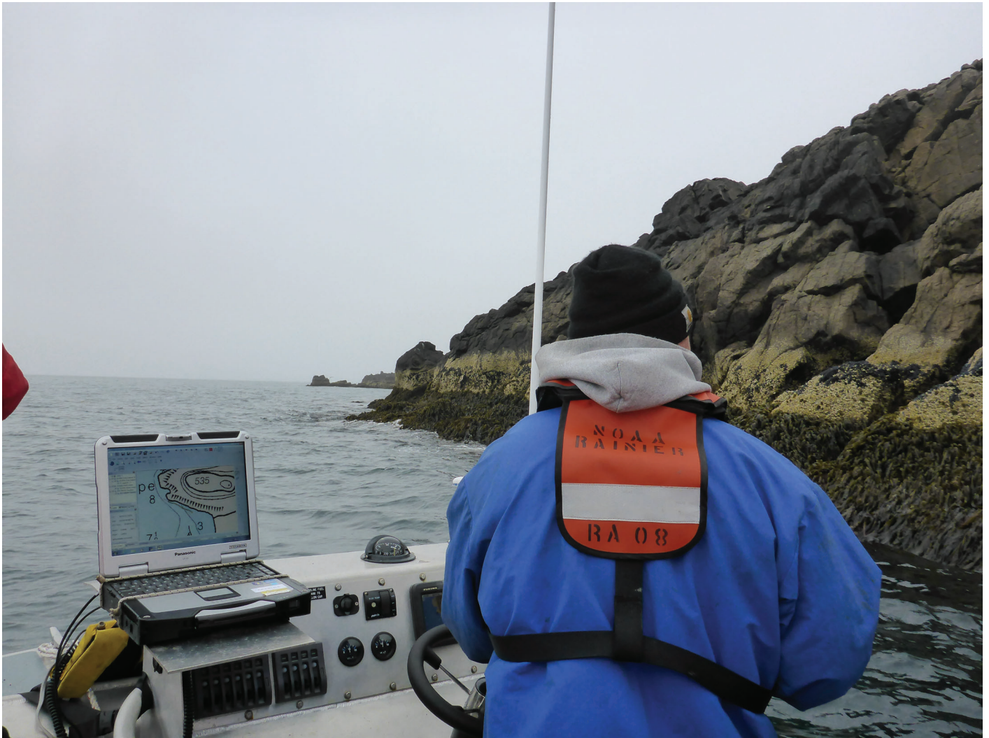
Figure 19: Survey skiff collecting the along-shore buffer line using a Trimble GPS backpack system connected to an external battery and a Toughbook computer.
