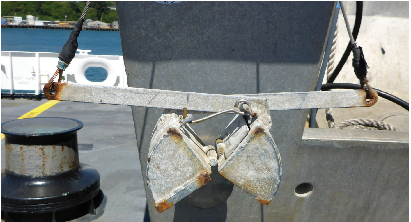
Figure 17: The Van Veen grab sampler configured ready to deploy.
