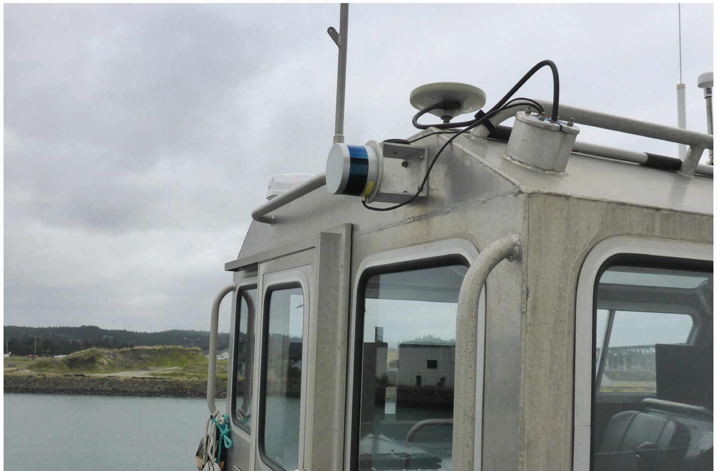
Figure 11: The Velodyne VLP-16 as mounted on 2701.
