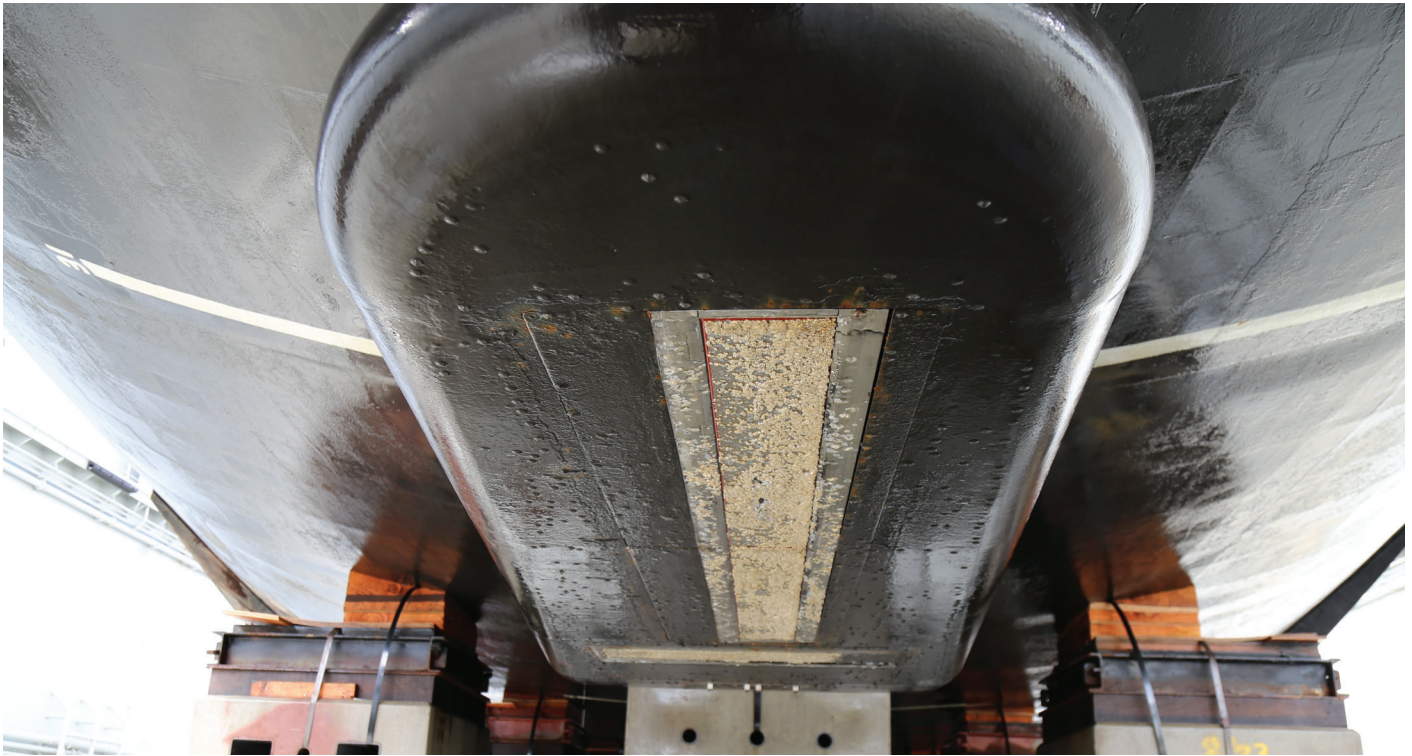
Figure 8: Kongsberg EM710 sonar transducer housing on Rainier (S221).
