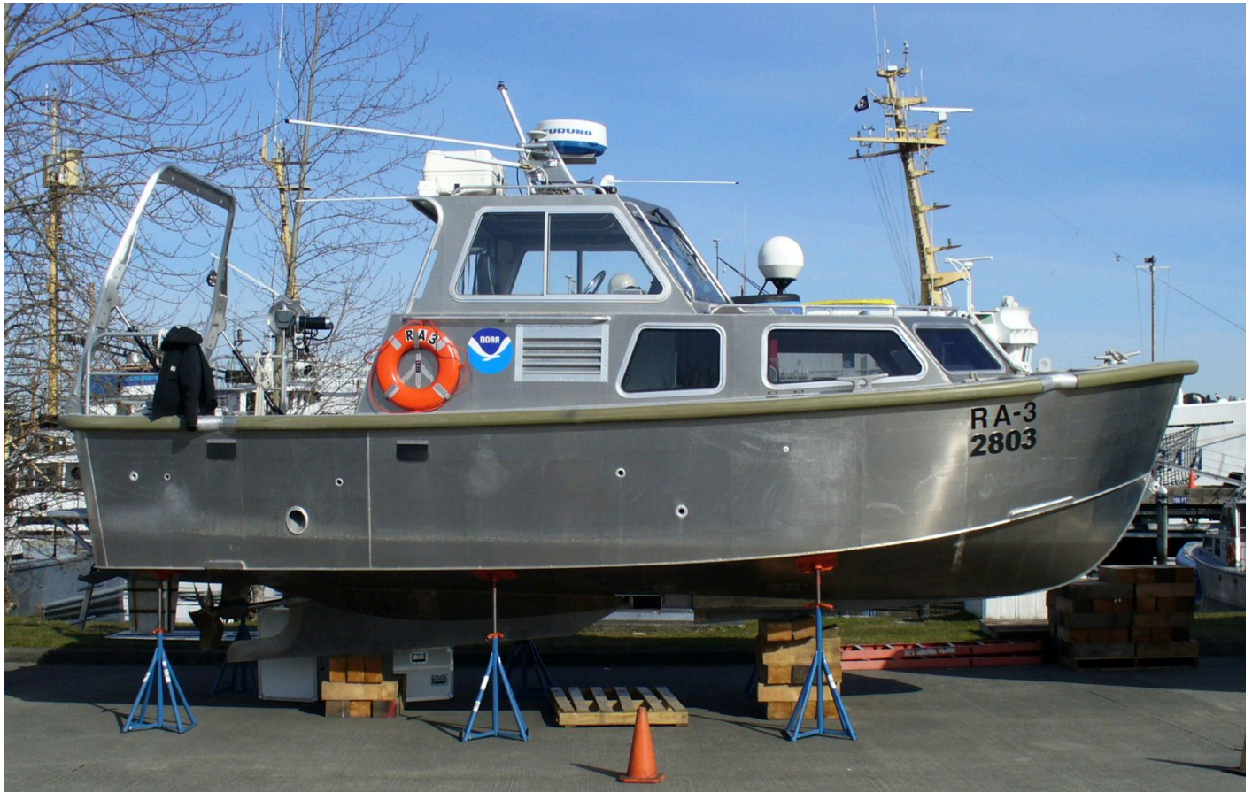
Figure 3: Rainier survey launch RA3 (2803) on blocks in preparation for her full static survey at Sand Point, Washington
