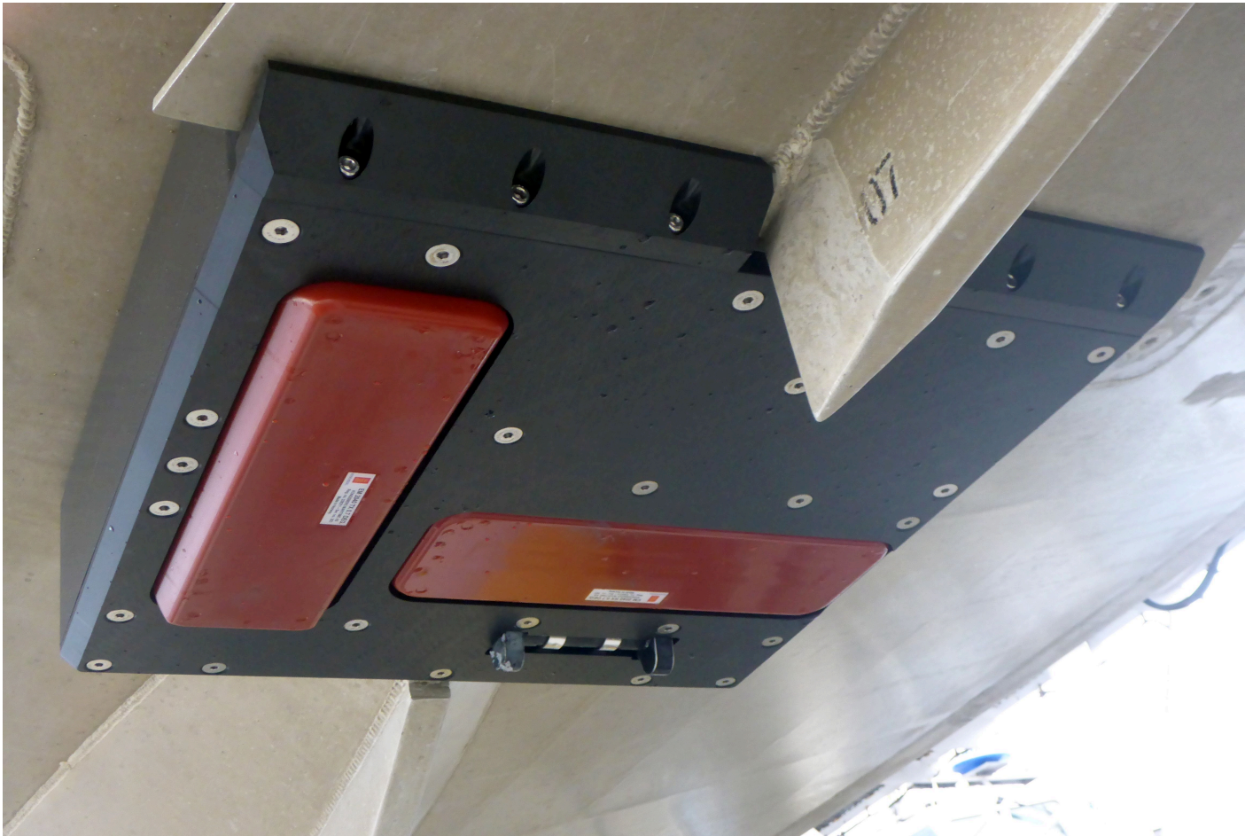
Figure 9: The Kongsberg EM2040-07 mounted on survey launch 2803.
