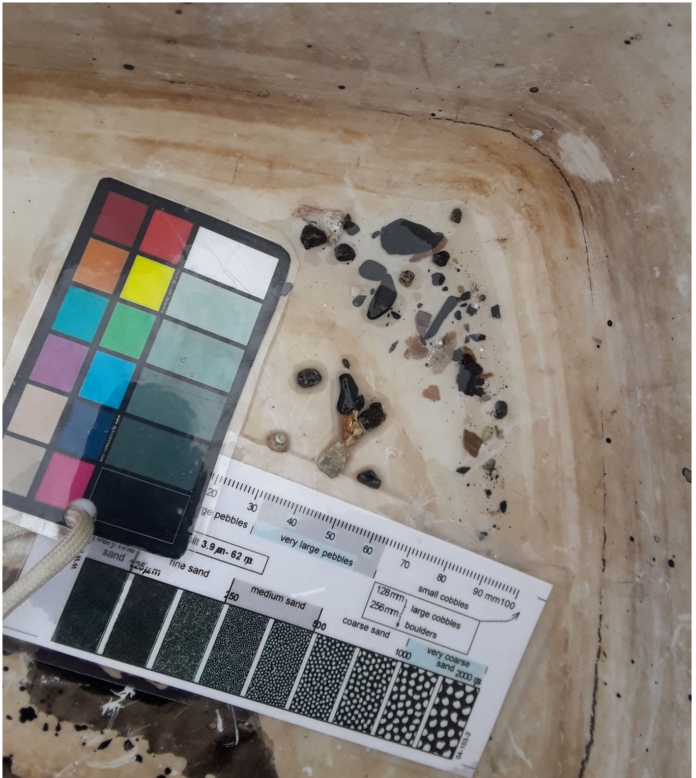
Figure 18: Bottom sample analysis using laminated cards with both color and size to classify a sediment sample
