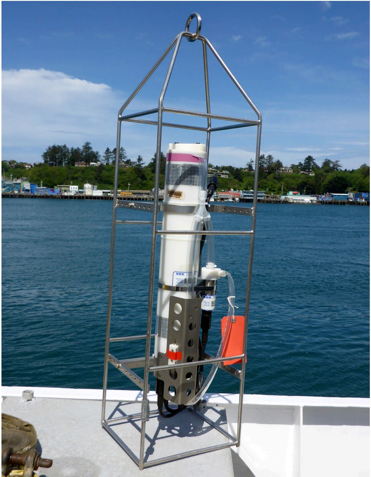
Figure 13: The SBE 19plus SEACAT profiler. Note the band of electrical tape around the housing at the top of profiler marking this as the "purple" CTD.
