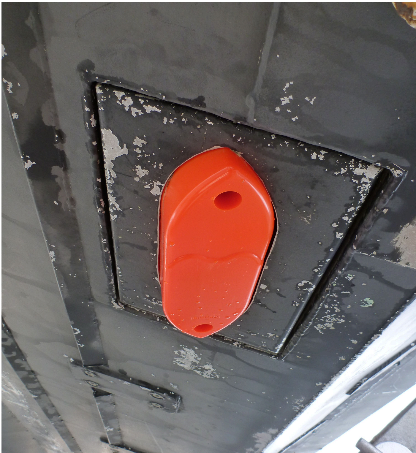
Figure 10: The Simrad 50/200 Combi D transducer as mounted on 2701 for the Teledyne Odom Hydrographic Echotrac CV200 hydrographic echo sounder.
