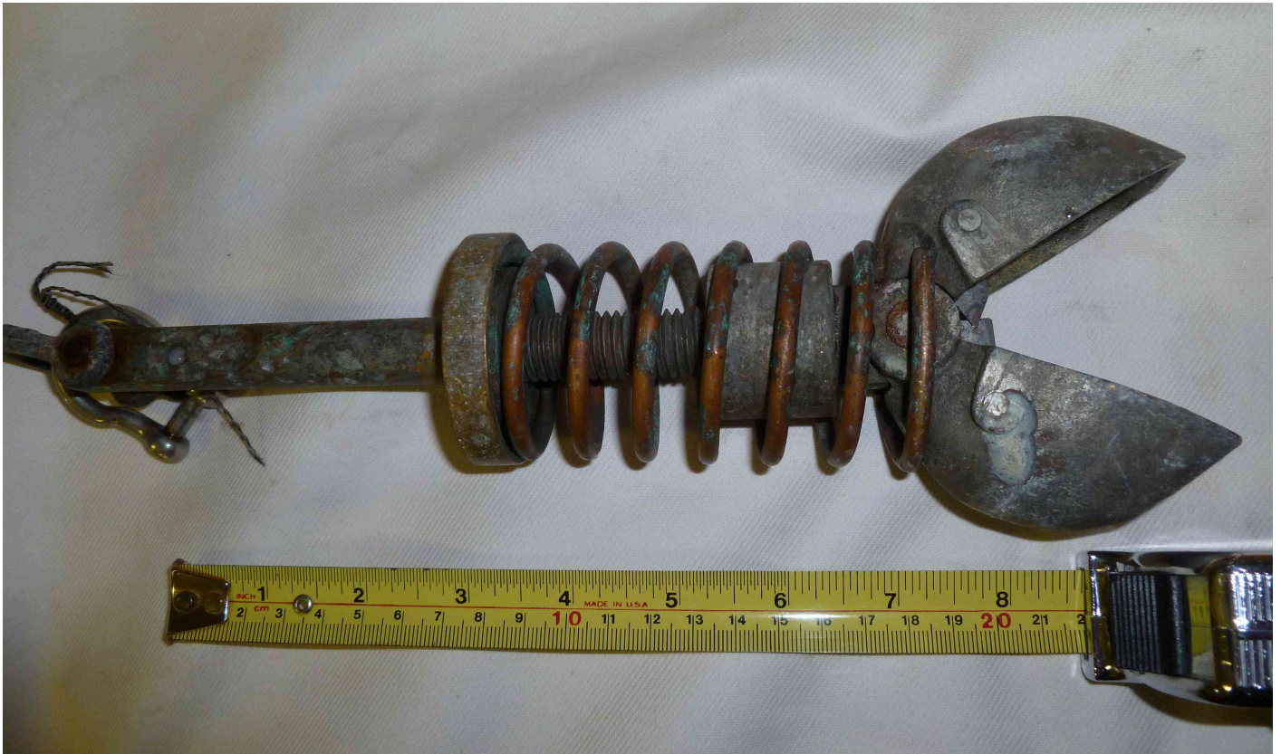
Figure 17: The “Nibbler”, a foot-trip clam shell style bottom sampler.
