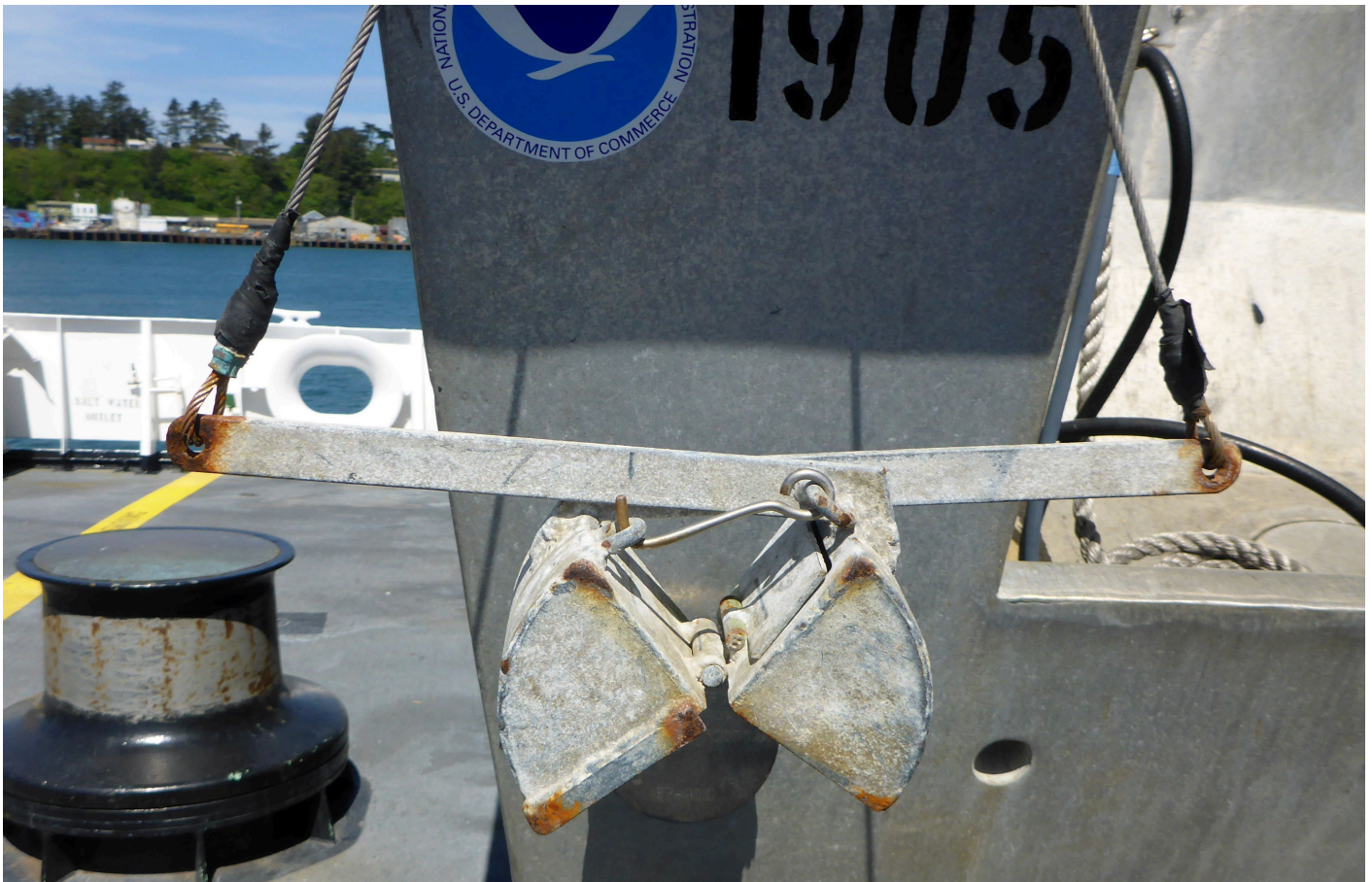
Figure 16: The Van Veen grab sampler configured ready to deploy.
